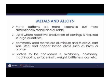
For repetitive production of casting in large quantities you can use them because they are, they are having larger strength, and the durability is more. Commonly used metals are aluminum and it is alloys, cast iron, steel and copper based alloys, such as brass, and bronze these are the normally used alloys, which are used for pattern materials. The factor to be considered is availability, castability, machinability, surface finish, weight, brittleness, cost etc like.
