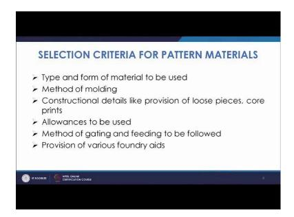
Construction details like provision of loose pieces core prints. So, when you take the, when you make the pattern, and if in the molding, you feel that molding cannot be possible, without the provision of loose pieces, in certain case you cannot make the pattern in a such a way that whole cavity is formed. So, sometimes you have to provide the loose pieces, this we will discuss when we talk about the type of pattern.
