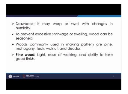
So, these are the normally used wood, which are used for making patterns, which are having that characteristic, which are suitable for making pattern material. You have the characteristics of all this varieties of wood, like you have Pine wood; which is Light, ease of working, and ability to take good finish.
