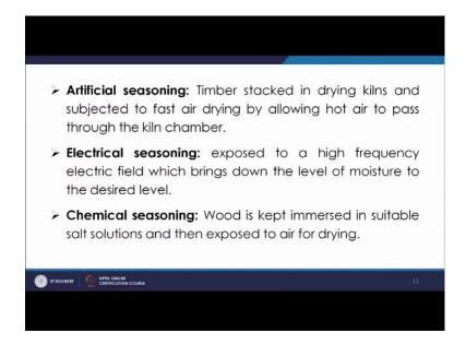
Electrical seasoning also is there, where it is exposed to high frequency electric field which brings down the moisture level quickly in no time. Chemical seasoning: where the wood is immersed in suitable salt solution and then exposed to air for drying, for drying so that the moisture content is kept under control.
