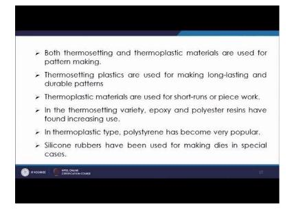
So, we have to use both kind of thermo setting and thermoplastic material. Thermosetting is certainly harder, then thermoplastics, and you have different varieties of thermoplastics and thermoplastics like in thermosetting variety you have epoxy, polyester resins, which are used in thermoplastics you have polystyrene which is mostly used we also use rubbers, silicone rubbers are also used, as pattern materials they are softer materials they are used for making even dice in this special cases.
