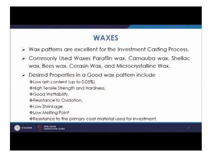
And most of the important property is Low ash content tensile strength and hardness should be better, Good Wettability, Resistance to Oxidation, Low Shrinkage, Low Melting Point, and Resistance to primary coat material because we are going to further first of all go for primary coat.
