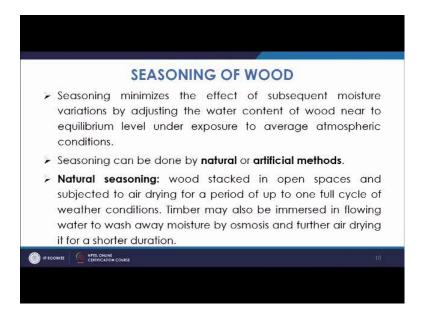
So, seasoning what it does, Seasoning is minimizing the effect of subsequent moisture variation by adjusting the water content of wood, near to equilibrium level under exposure to average atmospheric conditions. So, basically this is a process by, which we control this moisture content of water content. It can be done by natural or artificial methods. So, there are many methods by, which the seasoning is carried out.
