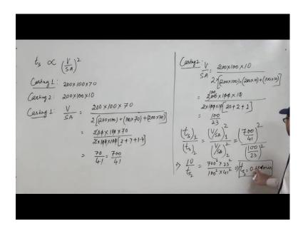
We have to calculate, the ratio of their volume upon surface area. If you take this as casting 1, casting 1 which has the dimension 200 by 100 by 70 and casting 2, have the dimension 200 by 100 by 10.
