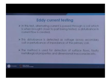
Now, what happens that you will have the primary coil and similarly when it will be brought to the cast the secondary coil is there? Now, if the there is no defect then there is no perturbance in that viscidity. However, if there is any kind of defect, then that disturbance can be seen. So, disturbance can be detected as the voltage across secondary coil or perturbance of impedance of the primary coil.
