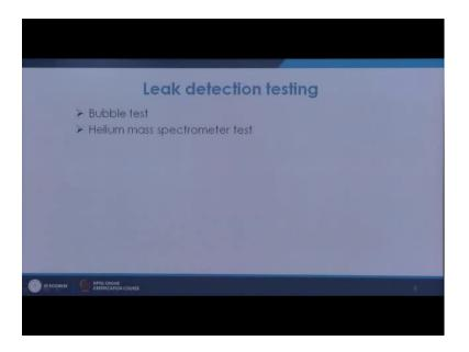
So, this way this bubble test is carried out, we may also use the helium or hydrogen based solvents and that basically, because they have lower surf extension. So, that also uses is used as the pressuring media and in that basically facilitates the formation of bubbles and that gives you indication of having any leak or taking the preventive measures to further see that there is no further any kind of micro porosity in the next castings.
