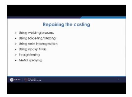
Then the straightening can be done if the metal has deformed and it has lost its shape because of many reasons, then this straightening can be done with the presses. So, either you are with manual or with the hydraulic presses or with mechanical presses, I mean it will be either mechanical or hydraulic. So, you have different kinds of presses you can apply the pressure and you can straighten the material is straight portions can be straightened if it is deformed.
