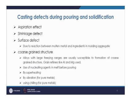
So, for that you have basically to have the proper design of the sprue system so that there is no aspiration. There is a chance of shrinkage defect because during the solidification process there will be shrinkage is going on. So, the shrinkage defect is also likely to occur and as we know that is to be compensated by placing the riser and there are many methods for calculating that. Surface defect become because of the reaction between molten metal and ingredients in molding aggregate.
