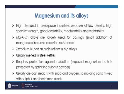
Now, this material normally is used as alloy that is Mg-Al-Zn, it is now largely used for castings. So, what happens? Small amount of manganese this material otherwise as very small corrosion resistance. So, if you add some amount of manganese it increases its corrosion resistance. So, this is further used for many applications.
