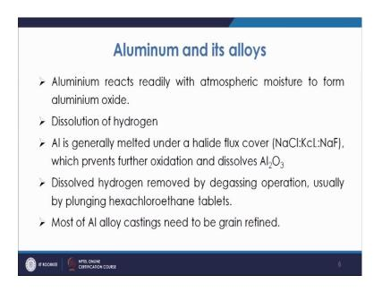
Then if you come to the aluminum and its alloys, so aluminum basically reacts very readily with atmospheric moisture to form aluminum oxide.
