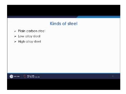
So, it is plain carbon steels where the alloying element is very small and then low alloy steels and high alloy steels which have the alloying content material content may be less than 8, then it is low alloy steels, high alloy steels you have more than 8, then in that case you have variety of steels like you may have the stainless steels.
