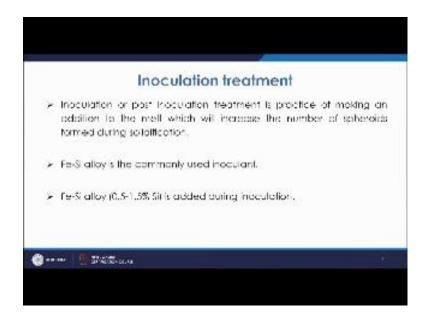
So, in this case the main purpose is to increase the number of spheroids and that is done by the inoculation treatment. So, normally the ferrosilicon alloy is the commonly used inoculants. So, 0.5 to 1.5 percent silicon is there, that is added during the inoculation and
