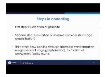
So, first step is the nucleation of graphite and the second step you are elimination of massive carbides that is first stage of graphitization and second stage of graphitization, in that case what happens once you slowly cool through allotropic transformation, in that case you have formation of completely ferritic matrix formed.
