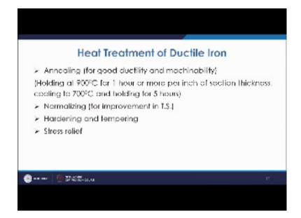
Now heat treatment of ductile iron; you do number of the heat treatment processes and among them are annealing, normalizing, hardening and tempering and also stress relief. So, annealing will be done for getting the good ductility and machinability that is done by heating at 900 degree C up to that holding for one hour and then further even more one hour plus for again one hour per inch of section thickness and then you are cooling to 700 degree C holding for 5 hours then further cooling.
