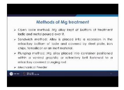
Now, in that case you have open ladle method. So, in the open ladle method magnesium alloy will be kept at the bottom of treatment ladle and metal is poured over it. Now as we know magnesium burns very quickly, it oxidizes so quickly. So, the reaction is volatile.
