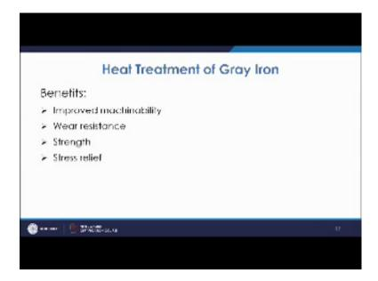
So, the properties which can be improved by the heat treatment process are the improved machinability, wear resistance, strength and stress relief. So, as we know that forgetting the improved machinability you will have to go for (Refer Time: 29:07) treatment where you heat and then you are cooling or you are holding in the furnace and then cooling slowly. So, in that case your machineability is improved it become soft.
