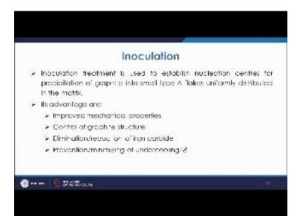
So, it is used to establish nucleation centers for precipitation of graphite into small type A flacks uniformly distributed in the matrix. So, basically you have the nucleation of graphites and for its better flacks and type A flacks this in occultation treatment is done. So, what happens if you have the better in occultation treatment and better nucleation of graphite, better type A flacks are formed in that case you are getting the better mechanical properties.
