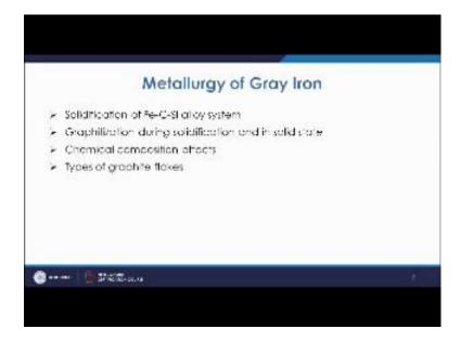
So, we will discuss in brief the solidification of iron, carbon, silicon, alloy system because as we know that although the grey iron or the cast iron is normally of iron and carbon but already we have discussed that silicon is one of the prime alloying element which basically controls the graphitization process. So, we will discuss the iron carbon
