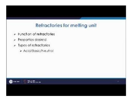
And neutral normally is your conium is used as the oxide is their which is used as the neutral refractories. Apart from that we have other refractories also which are neutral. So, this way you have different kinds of refractories which are used in the furnaces depending upon the requirements, depending upon the type of slags which you are likely to get you use the different kinds of refractories.
