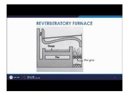
So, it has a large long shell and in that the blowing is from one side and then that because of that combustion products and because of the temperature of the flame, this heating takes place from the side of the walls which is refractory and then the heat and this is basically used for small scale foundries, where a small quantities of metal is required mostly for non ferrous materials.
