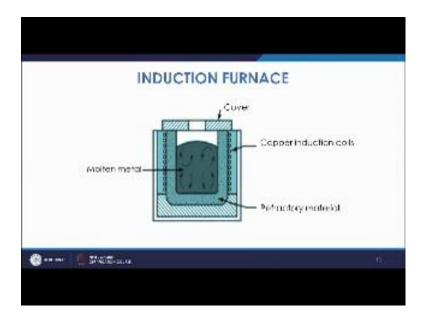
So, then comes the induction furnace. So, here what happens there is induction effect. So, what happens you have the primary coils these copper coils are there and when the oonj around this reservoir, and then once the electricity is passed so because of the induction effects, the eddy current is generated in the this charged material and because of this eddy current large amount of heat is generated.
