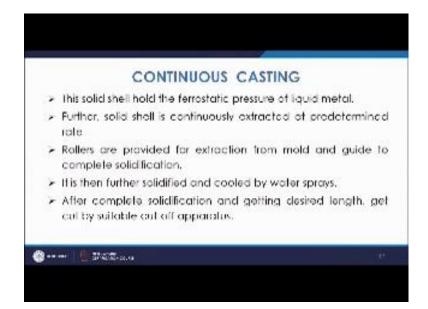
So, solid shell holds the Ferro static pressure of the liquid metal, and then it is continuously extracted at predetermined rate. Rollers are provided for extraction of from mold and guide to complete solidification and then it is further solidified and cooled by water sprays and after certain length it is getting cut.
