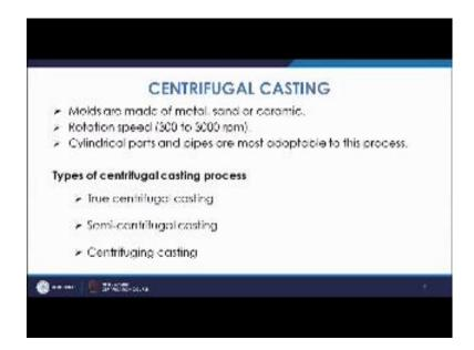
Molds are made of metals and or ceramic. So, the mold may be made of either metals or ceramic which is rotated at a speed, which is ranging generally from 300 to 3000 rpm, cylindrical parts and pipes most adaptable to this process. So, these cylindrical parts and pipes are normally manufactured using these processes. The different varieties of the centrifugal casting are true centrifugal casting, semi-centrifugal casting and centrifuging casting.
