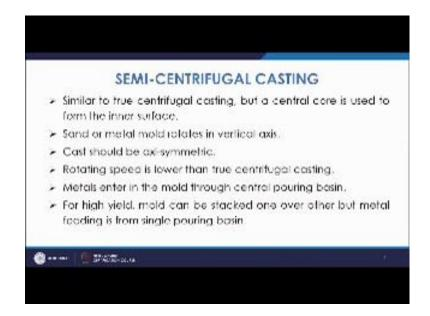
So, in that basically the advantage is that you can produce more complicated shapes because in this case the shape is very much simple you can produce, but if the shape is going like this and this. So, in that case that cannot be produced by the normal centrifugal or true centrifugal casting. So, in this case those complex shapes also can be produced for axi-symmetric castings.
