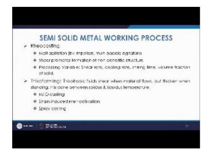
One of them is rheo casting. So, what is rheo casting basically? So, in that case what happens now in this case in this semi solid metal working process, the aim is to avoid the dendritic type of a structure and you try to see that you get favorably equiaxed global of the structures.
