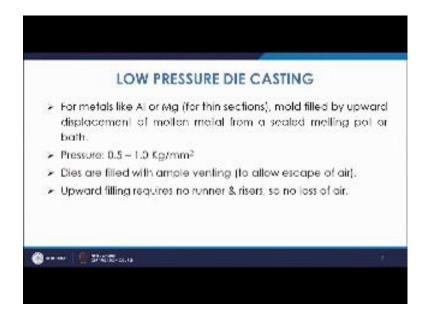
Now in this case the pressure requirement is less that is why it is known as low pressure Die casting. So, here the process is adopted in such a manner that the pressure requirement is less, now what happens for metals like aluminum or magnesium, the requirement is felt only because when you apply large pressure, then there is possibility
