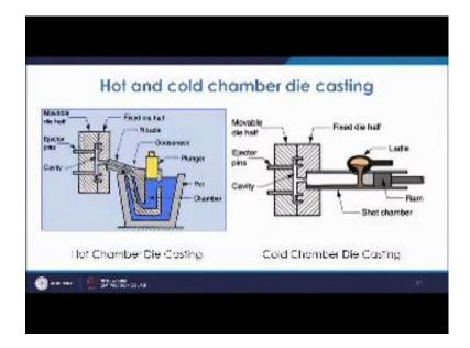
So, in this case in the hot chamber casting, this is a furnace, so you have heating you know arrangements, and the metal will be supplied from here. So, then once you apply this plunger, the metal will go from here and through this goose neck and it will be forced into this cavity and then it is this pressure is maintained.
