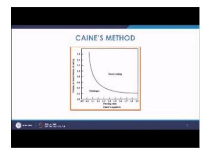
So, this freezing ratio is nothing but the relative freezing time of the riser to the casting, and that is y, this freezing ratio why this x is the ordinate, this is the volume of riser to volume of casting. So, this is x, x is volume of riser to volume of casting.
