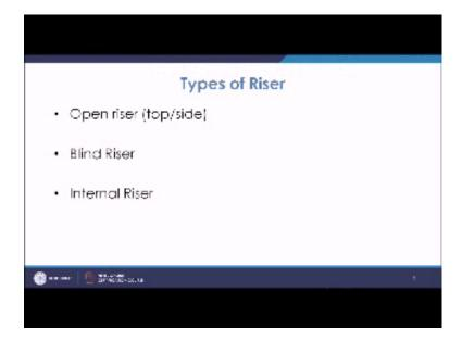
Types of risers, now you have the riser as we have seen in our first slide that you have to place the riser and it should be attached to the casting so that it should be able to supply the liquid metal to the casting whenever it is required. Now the type of riser is, one is open riser then open riser means the riser is open to atmosphere, the top part of the riser is open to atmosphere and there are 2 types of forces which are acting on this riser to feed the molten metal to the cavity.
