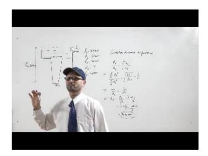
So, in this question, you have been given a pouring cup and a downsprue, then the downsprue length 180 mm. So, this length is 180 mm which is normally we take as h 2, then diameter of 20 mm at its top end. So, this point is point 2. So, here the diameter d 2, at this point you have d 2. So, h 2 is given as 180 mm, and d 2 is given as a diameter of 20 mm.
