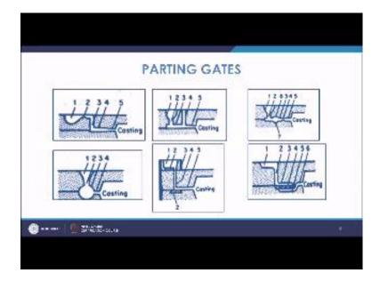
Now, if you look at this portion, in this case what we see here is this is the pouring basin, 1 is the pouring basin and in the 2, 2 it is basically a dam is made here so that all the heavier inclusions.
