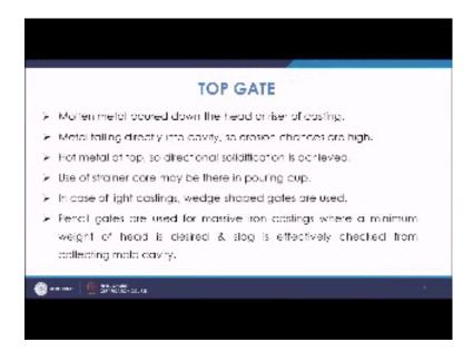
Basically you have the metal molten metal poured down the head or riser of the casting. So, what may happen that from the top itself, it has come and here from itself you can directly poured and you can directly pour and it may go into the casting. So, this is known as top gating. So, this may serve as a reservoir or a riser which can feed the metal in case of shrinkage.
