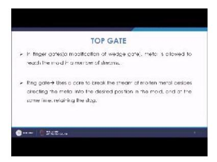
Then you have finger gate which is nothing, but a modification of the wedge gate and what metal is allowed to reach the mold in a number of streams. So, if you look at this finger gate. So, it is just like a will wedge gate, but you are allowing it to pass through a number of streams.
