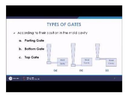
We have studied about the gating system and there the main purpose is to ensure that metal is fed to the cavity and the metal traversing the path by following the route from pouring basin from there it comes through the sprue goes to the runner and finally, to the gates and then it enters into the cavity.
