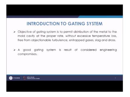
Objective of gating system is to permit distribution of the metal to the mold cavity at proper rate without excessive temperature loss free from objectionable turbulence entrapped gases, slag and dross.
