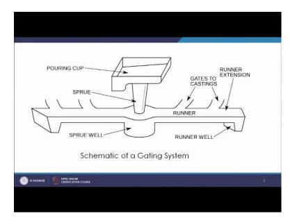
Let us see the schematic of a gating system. So, in the gating system you have a pouring cup or pouring basin now molten metal is coming here and from here it goes through this vertical channel that is known as sprue and it goes into this runner well sprue well it is basically and from this is sprue well, this liquid stream is basically directed towards these directions. So, this channel from this sprue well from where it goes in the directions this
