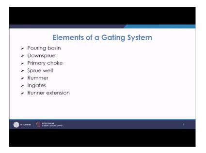
We have seen that you have these different elements of a gating system you have pouring basin. So, this is sprue, it is also known as downsprue then you have a choke, now this choke is basically the minimum cross sectional area in this channel which basically concludes the pouring rate. So, that is known as a primary choke, normally it is at the bottom of this sprue, but it may be at any other place. So, that is known as a choke because it is controls that is why it is known as the choke.
