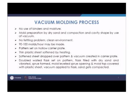
So, first of all the problem related to binders and moisture that is gone, the cost basically on the cost aspect also you can see the benefits then mold preparation is done by dry sand and compaction cavity shape by use of the vacuum. So, you have dry sand, the compaction or basically keeping the mold at its position, keeping the molding material or sand at its position. So, that you get the desired cavity shape, that is done by using the vacuum.
