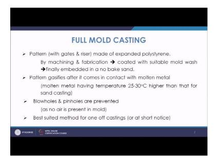
Now, this is known as a full mold means the mold basically has the pattern into it, when we are casting and we are trying to pour the molten metal into the cavity in normal circumstances the cavity is hallow, where as in this case the cavity is not hallow rather it is full. So, that is why it is known as the full mold casting.
