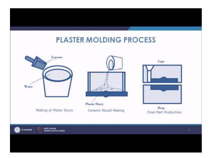
So, you can see the schematic you make the slurries, pour on this slurry on the pattern once you get these two halves, you have the portion from where having this scrucope and then you have the poring machine through which you pour the metal and it is comes and gets solidified. Now vacuum molding process the name indicates, that you use vacuum to make the mold and then the poring is done. So, in this case the advantage is that there is no use of binder and moisture.
