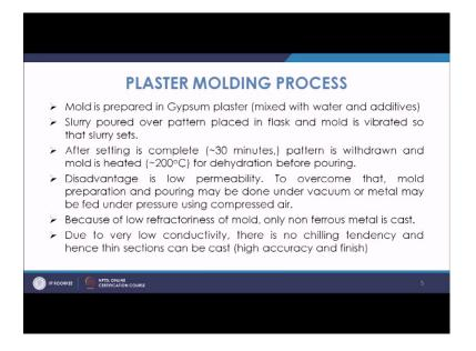
So, in this case you are preparing the mold with the gypsum plaster mixed with water and also we add the additives, so that you get the desired properties, I mean specific properties what we want to achieve. So, once you are mixing the gypsum plaster with water and the additives, this is in the form of slurry. So, this slurry is basically poured over the pattern.
