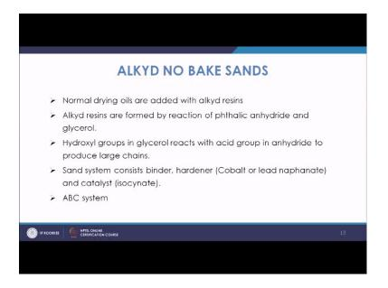
Then one or the other variety is alkyd no bake sands. So, in that case basically as the name indicates the baking is not required, in this case you use the normal drying oils. So, normal drying oils which are used for making cores that is known as core oil, now in that case you are mixing these oils with certain resins. So, that is known as alkyd resins. So, they are formed by reaction of phthalic, anhydride and glycerol.
