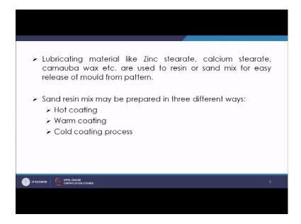
Now the sand mix is basically made in three different ways, so that coating of the resin on the sand takes place in 3 ways, one is hot coating, warm coating and cold coating process.
