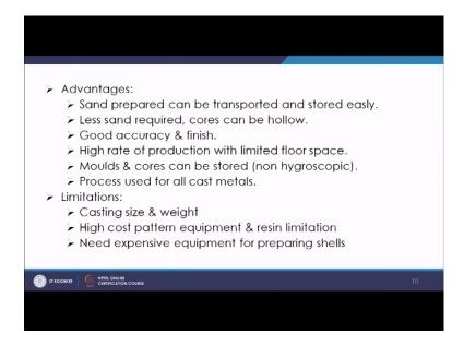
You have many advantages of these processes and you can see that sand prepared can be transported and stored easily you have less sand required, because you are making a shell which is very thin one and it as good sufficient strength.
