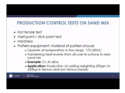
Now they are basically different tests which are done on this sand coat, and they are hot tensile test it is done at different temperatures or are different time may be 1 minute and 5 minute after that, similarly for melt point or stick point test, then hardness test. So, this way you do to ensure that your shell which has be made will come to the expectation of withstanding the pressures or forces of the metal.
