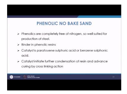
So, there is no probability of having any defects like phenol porosities. So, these phenolic resins are normally used as binders in such system which is free of nitrogen. So, catalyst is paratouene sulphuric acid or benzene sulphonic acid. So, this is the catalyst in these cases and catalyst initiate further condensation of resin and advance curing by cross linking action.
