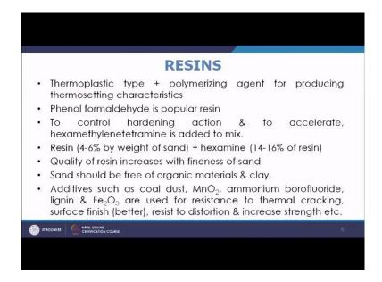
So, in this basically resin is thermo plastic type plus you are adding certain polymerizing agent, so that you get this thermo setting characteristic; normally phenol formaldehyde is the resin which is used. The control hardening action and to accelerate you are adding the hexa that is hexamethylenetetramine. So, that is working as a catalyst. So, that the hardening action is accelerated.
