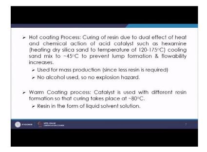
So, caring of a resin due to dual effect of heat and chemical action of acid catalyst such as hexamine, so heating dries silica sand to temperature of this and cooling the sand mix to 45 degree C to prevent lump for formation and flowability increases.
