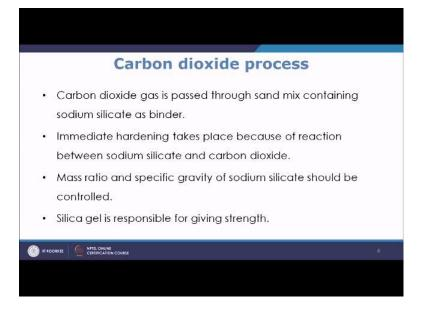
So, immediate hardening takes place because of reaction between sodium silicate and carbon dioxide. So, what happens the Co 2 in the case of this carbon dioxide process, the sodium silicate will react with carbon dioxide and it forms a hard response mass basically and this formation or this action of cohesiveness or the strength is because of the formation of a reaction product that is known as silica gel.
