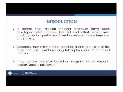
So, what we have so far studied, then we are seen that special molding processes are required to be developed, which require less skill because in the case of molding or core making in core making any way do not use the clay, but the molding while we use the clay, but in the molding while we use the clay you need a person with good skill and also the rate is not so fast and the effort is quite high, you need to have processes where so
