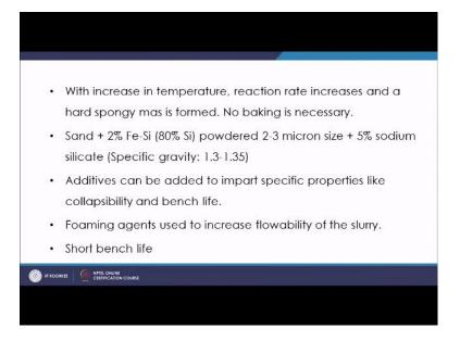
So, in this case what we do is, sand will be added with 2 percent ferrosilicon which has 80 percent of silicon in that ferrosilicon; which is powder 2 to 3 macron size. So,
