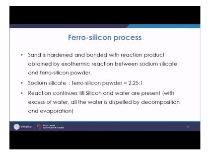
So, what happened here without use carbon dioxide gas to pass through it, so what happened here is we use this ferrosilicon powder; so once this ferrosilicon powder is used this reacts with this sodium silicate and this reaction is a exothermic reaction and in
