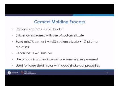
In that is you have sand mix 2 percent, cement plus 4.5 percent, sodium silicate plus 1 percent pitch or molasses to give the specific property and in this case you are getting the cement mold which has a bench life of 15 to 20, you can use the foaming chemicals, so that ramming requirement is decreased and the mold normally it is used for large molds large size castings and good seek out properties.
