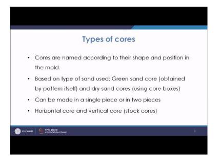
So, cores are basically named according to their shape and position in the mold. So, different type of shapes at different positions we use the cores based on that, you we give the different names. First of all depending upon the type of sand used we may have green sand core where the core is made of made by using the pattern. So, that type of coring known as green sand core. So, where you are making the mold cavity, that time with the
