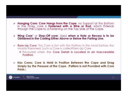
Then hanging core, now what happens sometimes we need to hang it, so no support at the bottom in the drag. So, basically in this case what we see is, this place is basically nothing, here you have metal. So, this way your structural will be like this and here it will be a straight line and then this way it goes. So, it is supported at the bottom, this type of cores have a support at the bottom whereas, when there is no support at the bottom in
