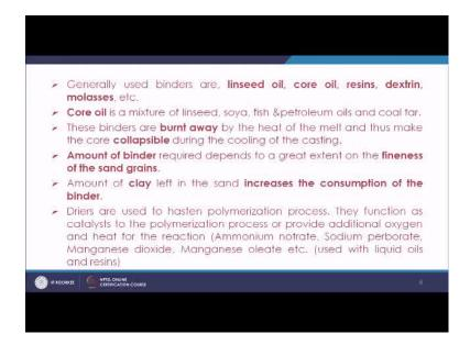
The generally used binder, are linseed oil core oil resins dextrin molasses etectra. So, these are the general used binders core oil is the mixture of linseed soya fish and petroleum oil and coal tar. So, basically this is the organic binder that is used for making the cores. So, these binders basically are burnt away, by the heat of the melt and make the core collapsible during the cooling of casting.
