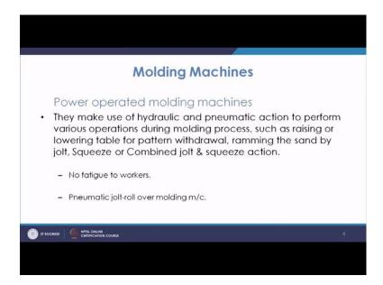
So, there are the power source, and the fatigue which is created to the operator in using these levers, in pattern draw and squeeze type or so, that is basically missing in this case. So, that you are getting rid of that fatal to the workers, and that increases the productivity of the worker.
