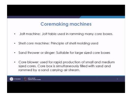
Next is the shell core machine. So, in this case, as it is written principle of shell molding is used. So, we will discuss about shell molding later, where in that case the organic binders are used and the sand when reacts with the organic binder and comes in contact with a heated metallic pattern or heated metallic sheet, the sand mixed with binder at that particular temperature sets, and it gives you certain thickness.
