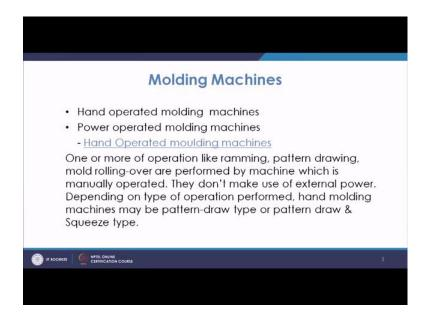
Now, molding machines are either hand operated or power operated molding machines. Hand operated means, now these both are the machines where main work is done by the machine, there will be a platform, on that the box is to be put in, the run input purpose is solved, running is to be carried out.
