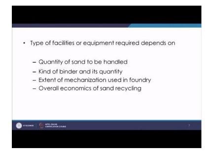
The factor is quantity of sand to be handled, how much quantity you want to handle, it is small or larger. Kind of binder and it is quantity, binder may be in organic based or it may be organic based, based on that this reclamation process will vary. Extent of mechanization used in foundry, foundry may be manually operated; mostly manual or it may be automatic semi automatic or fully automatic. And overall economics of sand recycling,
