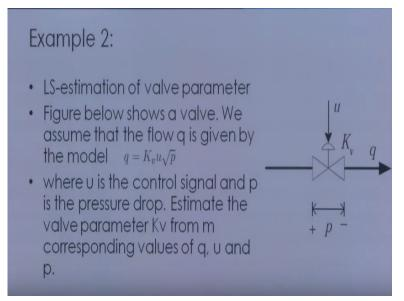
Now in this valve you can see that this is the direction of flow say a pipe okay through which a flow q and here is your valve all right. now in this valve there is a control signal u coming here okay and because of this control signals there is say when the say water passes through this valve okay. There is a drop in pressure p okay.
