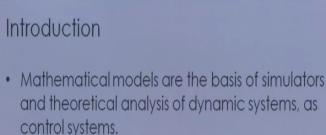
• The model can be in form of differential equations developed from physical principles or from transfer function models, which can be regarded as "blackbox"-models which expresses the input-output property of the system.
