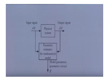
So this is what we are going to see in this lecture that how can we identify through this estimator for mathematical model by giving the input and output signal. How can we modify measure the model parameters. So here in this lecture we will discuss the popular least square method or in short or what is called as LS method for the parameter estimation okay.
