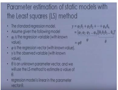
So for this actually are the standard regression model use and we can assume a model as it is indicated here or we can assume a model say Y = Phi 1 theta 1 okay + Phi 2 theta 2 and so on + Phi N theta N theta and all right. Now here what we do we segregate the Phi's and we segregate the thetas.
