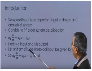
So this is what we are going to see today under the heading what we call it as frequency response and our aim of here is to see if my dynamic system is subjected to a certain sinusoidal input, what the output is coming okay or how the output, what is the output of it, okay, so as I said sinusoidal input is an important input in design and analysis of systems and say if you take a first order system.
