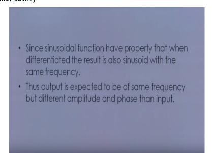
So you can see that this differentiation also has got the same frequency as that of the input, of course this amplitude has been changed, so thus output is expected to be of same frequency, but different amplitude and phase than input is there ok, so this is what is going to be and we can
