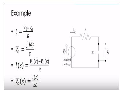
In order to complete the block diagram for the whole system. Let us take an example suppose this is a RC circuit okay and to this RC circuit there is you say applied voltage Vi and say I am interested in finding out the observing the voltage across the capacitor say Vo, so first step that we write the dynamic equation for the system.
