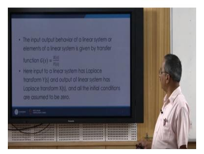
It indicates more realistically the signal flow in a system. So suppose the input output behavior of a linear system is given by a transfer function see gs=Laplace transform of the output/the Laplace transform of the input, here as I said input to a linear system as Laplace transform ys and the output of linear system has Laplace transform xs okay.
