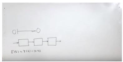
So and here you can see that the output the output of this block diagram that is access is being fed here okay. To the summer to find out the error, so this type of block diagram is what is called as the closed loop system okay. You may ask a, you may ask some practical example or why we are going for this closed loop system or what is the practical example of this closed loop system? so let us look at this figure.
