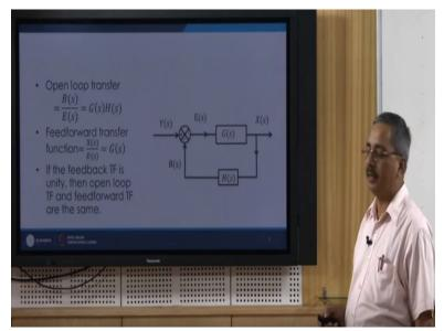
If the feedback transfer function is unit, then open loop transfer function and feed forward transfer functions are same. So you can see that if I put this as unity, unity then whatever are we get here this and this both are going to be the same value okay. Next is the closed loop transfer function now this closed loop transfer function is basically defined as the ratio of Xs/Ys okay, so to get the derivation for the closed loop transfer function okay.
