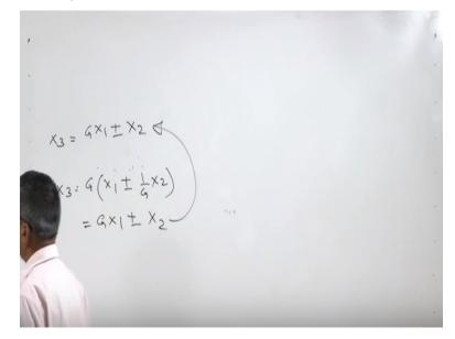
In the case or the second figure what we will have is X3=GX what we have X1+-okay, we will have 1/GX2 okay or this is a GX1+-X2. So this is same as this one that is why both these blocks are equivalent blocks okay and this one we have already seen that I am in case of a closed loop system okay, so in case of closed loop system the overall transfer function between the output and input is given by here X2=here X2/X1 is basically GH upon 1+GH okay.
