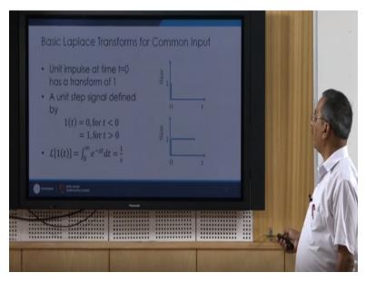
So let us see the basic Laplace transform for the common input okay, suppose first we have the unique impulse at time t=0, so here if I plot the size versus function of time the, so here at 0 time, I have got a unique impulse okay, so the unit impulse at t=0 has got Laplace transform of 1 okay, similarly I can define a unit step signal defined by say1t=0 for t less than 0 here, this is 0 and this value is 1 for t value greater than 0 okay.
