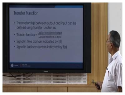
So these differential equations can be converted into an algebraic form using Laplace transform okay and what we say that the conversion has taken place from the time domain to S domain okay, time domain is usually differential equations are written in the time domain and of course the Laplace transform is carried out in the complex domain or what we call it as the s domain okay.
