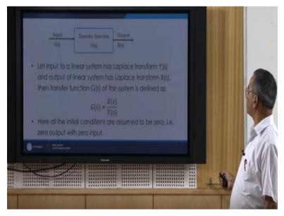
So here you can see that suppose we have a transfer function say Gs and input to the transfer function is Ys and output for the transfer function is Xs then we can define this transfer function Gs as ratio of Xs and Ys okay. So of course this is valid for a linear system and as I said if the linear system has Laplace transform Ys that is the input to the linear system as Laplace transform Ys and output of the linear system has Laplace transform Xs.
