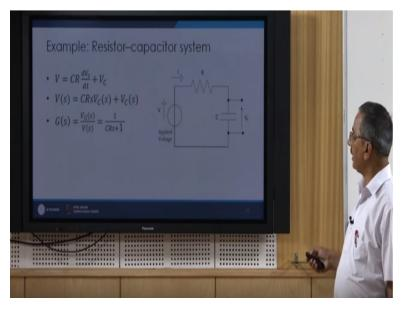
We can take the example of a physical system say resistor capacitor system here okay. Now in this case say resistor is represented by R and capacitance is represented by C and say the applied voltage is V and my interest is to find out the voltage V C that is V C is the voltage across the capacitor so that is my output okay. So using the Kirchhoff's voltage law, I can write the system equation as this one okay that is the loop equation for this loop.
