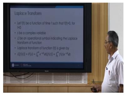
So let us see what the Laplace transform is okay. So let Ft be a function of time F be a function of time t such that Ft=0 for t less than 0 that is for the time value less than 0 the function value is 0 and sba complex variable then we can use this Laplace operator this symbol as operational symbol indicating the Laplace transform of the function okay and thus Laplace transform of a function Ft is given by this one.
