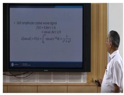
Likewise, we can find out unit amplitude cosine wave signal okay, so for cosine wave signal I can find out Laplace transform that is I define the cosine wave signal Ft=0 for t less than 0 and for t greater than or=0. We have this as cos omega t okay so the Laplace transform for this will
