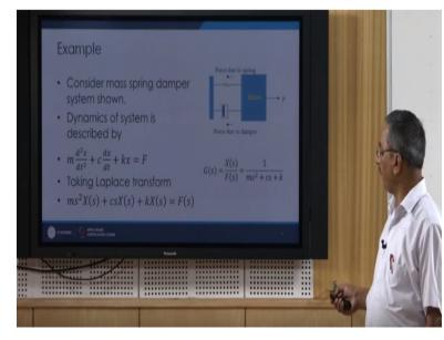
Now let us take an example of the transfer function okay so here I just take a simple spring mass damper system let this end of the spring and damper is anchored to the ground and other ends are anchored to the mass okay and here say stiffness of the spring is k and the damping constant of the damper is say c and let the mass be small m and a force F is being applied here.
