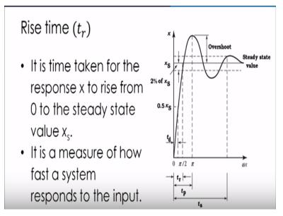
So, this is how we define the delay time next time is the rise time okay and you can see in this figure that this is that vice time represented by tr and this is basically the time required for the system to reach up to the steady state value okay.
