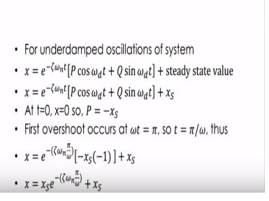
So, for under damped oscillations of the system we have seen in our last class that is last lecture that we can give the under damped oscillation of the system the amplitude x output is given by this relationship okay +the steady state value, so but basically this portion corresponds to that transient behavior add this is the steady state behavior okay our value corresponding to the steady-state.
