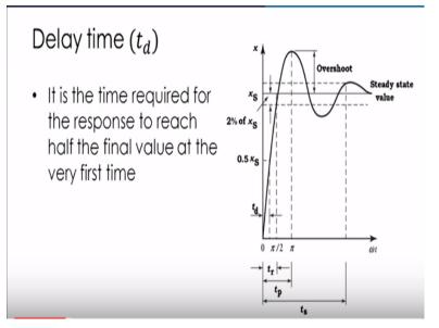
So, second order under damped system subjected to step input so in this behavior we can see that there are various parameters as I talk to you has been defined the delay time tt is basically this that is this parameter that is the td and it is the time required for the response to reach half of the final value at very first time okay so half of the final value final value means basically we are talking about the steady state value okay.
