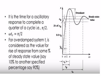
But as I said for the under damped system we define it as the time taken for the system to for the output to go from 0 to the steady state value. Next is the peak time now if you look at this plot you can see that this is the maximum value of the response x which the system could reach okay, so actually the peak time corresponds to the time okay by which the system attends the peak value okay.
