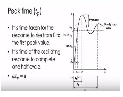
As I said it is the time taken for the response to rise from 0 to the first peak value and this is how it is defined and it is the time of the oscillating response to complete one half of the cycle so we write here Omega pp = pi and from here we can find out the pp value ok that is pi/Omega then next parameter is maximum overshoot mp okay which is represented in short form by mp.
