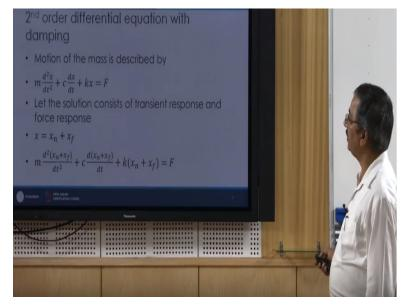
So again here I am going to consider the case of free vibration, so I am assuming this F to be =0 and since I am assuming there is no damping, so I can make the c term also =0 and whatever resulting equation will be md square/dt square+kx=0 okay, now let us assume that the solution for this is like this, x=A sine omega nt, where A is the amplitude of oscillation and omega n be the angular frequency of the free undamped oscillations okay.
