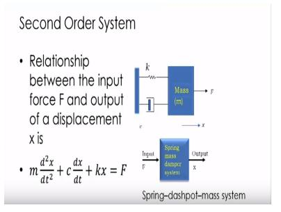
Let us take the example of the second order system okay, so also we say a spring mass damper system okay, this spring has stiffness k, the mass as mass of m and damping coefficient of the damped say c and say there is a force F being applied here and there is a displacement X of the system. So, here the input is F that is the force, which is being applied on the mass and the output is X for this spring mass damper system okay.
