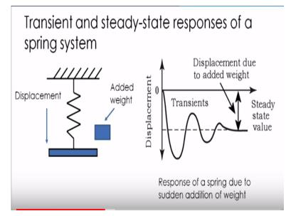
Let us take an example suppose, I have got a spring here and say there is some hanger here where I can aid up a weight okay. I say about the displacement of spring takes place in this direction. Now what happens initially there is no weight on the hanger which is attached to the spring and after some time I add a way to it. So what I am doing I am changing the input initially the input is 0 and then the input is that of equal to the weight.
