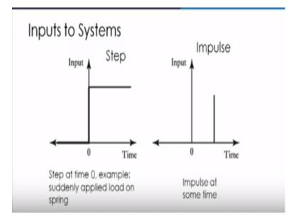
Now the previous example, which have seen that is adding up the weight on the hanger what it is basically it is a input to the system okay. It is the input to the system alright and that type of input. What we call it as the step input that is initially the value is 0. And then a definite value is given so this type of input is what we call it as the step input okay. We need to know the various types of inputs for which the system is subjected to in order to know the behavior of the system okay.
