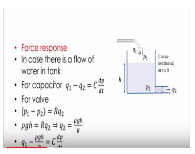
Then we could have a condition, where there is a tap with certain water coming from the tank and into the tank okay and then the response of the system whatever will be there that we call it as the force response. Fine, in this case there is a flow of water in that tank and we have already seen this derivation when we were discussing with the hydraulic system. I just want to take you to the first order differential equation in case of force response okay.
