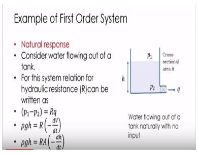
Suppose first we consider the natural response. Natural response means that here there is no input okay, so there is no path filling this tank okay. So in that case let us see how this h varies okay. So for the natural response okay, as I said consider the water flowing out of a tank and for
