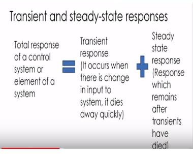
Then let us see the total response of the system. Now if I talk about the total response of the system it could be basically could be divided into divided as the summation of the 2 response okay and these summation are first one is the transient response and the steady-state response. Now transient response is basically it occurs. when there is change in input to the system okay, as the name indicates the transient response died out after some time okay.
