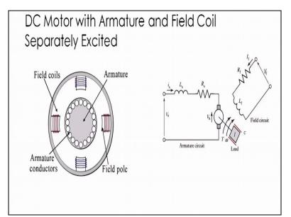
So let us see dc motor with armature and field coil separately excited so this figure shows you the dc motor this is the armature and this an armature conductor through which the armature the current passes. And here we have the field poles and a field coils are there and are this coils and responsible for the generation of the magnetic field b. So here I can just draw is schematic form of this motor here.
