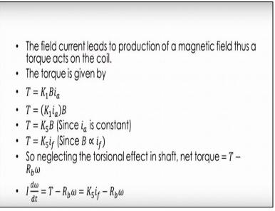
This torque given by k1 bia .now you see that i here since we are going to change the v because why we are going to change the v because here i am changing the current i am going to sorry i am going to controlled by the varying field voltage armature current is held constant. So here my b is changing and armature current I a held constant. So what I can do it that this k1ia I can make it constant into b.
