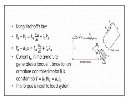
Now using Kirchhoff's law for the armature circuit I can write the v a - v b is equal to la d I a by d t + I a r a so this v b is the back emf and this is the voltage applied alright. So this is this will be the net voltage and this is going to be equal to la d i by d t + I a r a. Now here you see va known to us are this is the one which we are going to apply and vb we have just found out he k 3 into omega assuming b as constant. So here this is k3 omega and this la d i by d t + I a r a.
