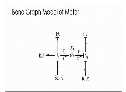
As per the gyrator relationship and here of course you have the load and here you have the bearing the resistance. So if you able to draw this bond graph you automatically get those two system equation one at which option in the previous line. next let us move to the field control motor so the previous case the previous case there we assume that if that is field current to be constant now in this type of motor armature current is held constant.
