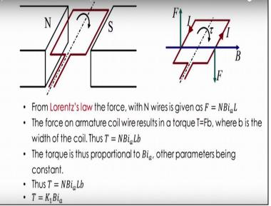
So, I take example of the magnetic field created by a permanent magnetic. Here the North Pole and the south pole of the magnetic and here is the current carrying conductor is placed. Now the Lorentz force law we can find out the forces if there are such wires here that will be just multiplication by n and of the forces which was generated in the single conductor.
