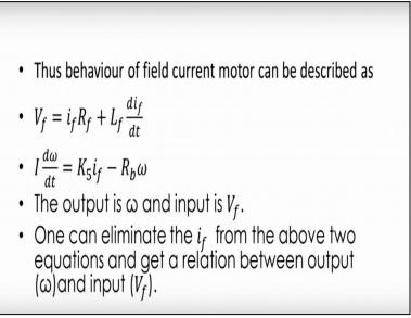
So the output here you can see that it is omega and input is v f .so again if I want to have the relationship between omega and the v f what we can do is that again we can take the Laplace transform and convert this differential equation into the algebraic equation and get it relationship. (Refer Slide Time: 32:43)
