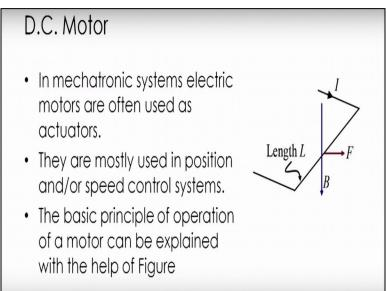
The basic principal of motor can be explain all of you studied in your school as well this basic principal that is current carrying conductor when it is places magnetic field there is the force on the conductor.
