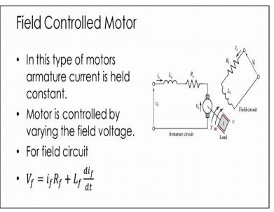
So basically armature current is held constant in this type of that is field control motor and this motor is control by varying the field. Voltage so here you can see for the field circuit again using Kirchhoff's law I can write v f equator that is total supply voltage v f equal to I f r f + 1 f dif by d t. And what field the current leads to production of a magnetic field the toque act set on the coil.
