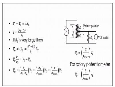
Now here you see that these voltage is v i and of course the voltage here is going to be v o, output voltage so if I apply the Kirchhoff's law here so this v i - v o going to be the i r 1 here. So I can find out the value of i from here that is v i - v o upon r 1. Now if we take r 1 that is resistance of the voltmeter at very high as I said in the begin itself. I can write v output v o as i into r2 or I can substitute for this i this is going to be equal to v i - v o upon r1 into r2.
