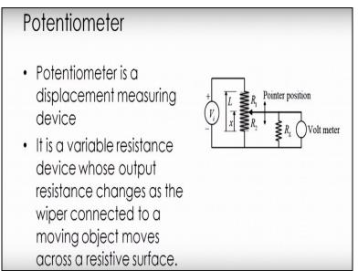
The potentiometer as I said is a displacement measuring device and it is a variable resistance device, whose output resistance changes as wiper connected to a moving object moves across a resistive surface. So here you can see that as this wiper moves across this rustle surface, the resistance changes and based on theses linear motion of this we get the electrical signal or we get the voltage here.
