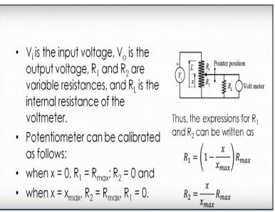
So, in this figure you can see that v i is the input voltage v o which is not return. Here v o is the output voltage and r 1 is and r 2 is variable resistances. And r 1 is the internal resistance of the voltmeter which we usually take to be of very high value. Now we can calibrate a potentiometer as follows. when x is 0 when this x is 0 r 1 is r maximum because this pointer will be at the position. So our r 1 will be r maximum and at that position r 2 is going to be 0.
