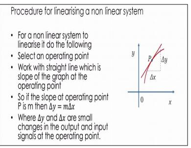
That is here suppose this is by output versus input curve for a system. And as you can see the behavior of this curve its a nonlinear curve. So, to analyze this or linearize this actually is done is that we select an operating point. Here, i am selecting the P as the operating point.
