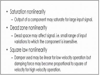
Saturation nonlinearity output of a component may saturate for large input signal. So if the input signal is large then the output may saturate it may not vary at all for the given input. So this type of nonlinearity as I said we call it as the saturation nonlinearity.
