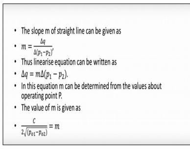
And the value of m as i said that we can get here Is equal to c by this value so i can get the one here and when i substitute this m value I get the linearize equation.
