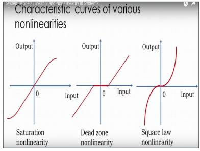
The first one you can see that with increase in input the output also increases. But after a certain value of input there, output remains almost constant and this type of behavior is call it as the saturation nonlinearity. Other type of nonlinearity could be the dead zone nonlinearity. If we lo at this graph now here in see that for a certain value of input there is no response for the output we don't have any output response and of course after sometime output changes with increase in input.
