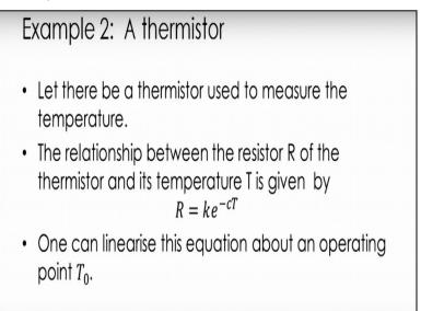
You can see that there is a exponential variation here you k and c are the constant and t is the temperature. Now I can linearizes an equation about an operating point t 0. So what happens, then the slope of the graph of r verses t at the operating point can be given by this one. That is I just differentiate this previous equation I differentiate this equation and I find out the d r by d t are the slope and this is the slope.
