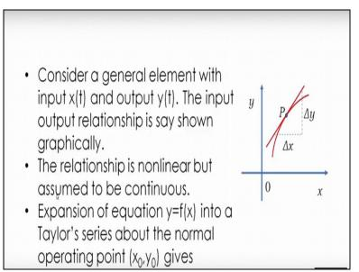
Now what we can do is that we can expand by the equation y=fx into a Taylor's series about the normal operating point x0 y0. Now if i do that this is what i am going to get the Taylor's series expansion.
