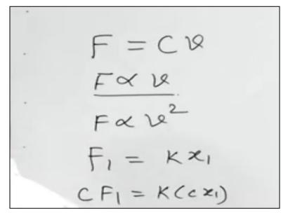
So, the thing is that if you have F1=k x1, and then if I multiplying here so cf1 will be basically k times cx1. This is what I mean by so these two conditions are fulfilled by a linear system. So let us see graphically this suppose we have a spring linear is spring and if I plot the force verses is x here then you can see that F=k x which is the characteristics for the spring and F1=k x 1 and f2=k x 2 then if i combine the f1+f2 i should get k(x1+x2) likewise if I put cf1 should get c times kx1.
