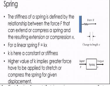
Let us begin with the first basic element that is spring now you see that we have schematic here being represented a spring is being represented and say force f is applied on this spring and because of this force there is a change in the length. Here in the block diagram mode I can just represent it like this, that there is an input f here to the spring and because of this input there is certain output x.
