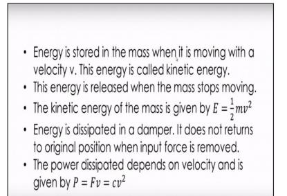
Now, energy stored in the mass when it is moving with a velocity v and this type of energy what we call it as kinetic energy and it expression all of us know that, half of the mv square where m is the mass and v is the velocity.
