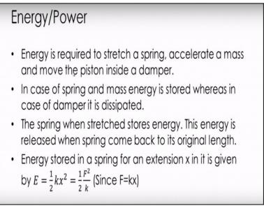
Now coming to the energy power, energy is required to stretch a spring, accelerate a mass and move the piston inside the damper. Now you see in case of spring and mass energy is stored whereas in case of damper the energy is dissipated.
