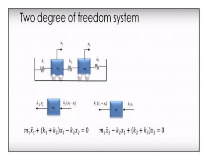
We can take by little complicated system like this here so two degree of freedom system now these two degree of freedom system there are the two mass which are the two connect by spring of the k1 k2 and k3 .so here what we k2 we take a direction a save positive direction x1 like this x2 like this.
