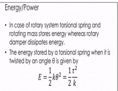
Then coming to the energy or power in case of rotary system, in case of rotary system tortional spring and rotating mass stores energy, whereas rotary damper dissipates energy the behavior is same. The energy is stored by tortional spring when it is twisted by an angle theta is given by half k theta is square or I can substitute for theta here I can get i half tou square by k. Similarly.
