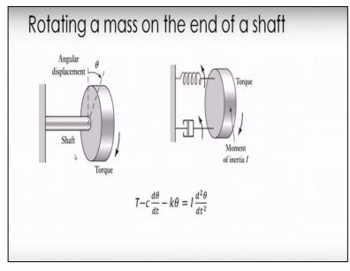
The last example I am going to take its rotating a mass at the end of shaft suppose here in the shaft here and this shaft at the shaft at the of there is the mass here and I want to represented are mathematically model is system .
