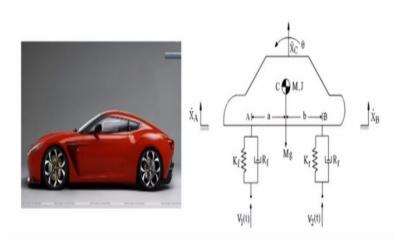
So this car is my physical system and I can convert this physical model of the car into an engineering model. As you can see in this figure of the car sidewise; the front and the rear suspension I have put into a car body having the car mass and the car puller movement of inertia and the vertical motion as well as the pitching of the car has been in physical model.
