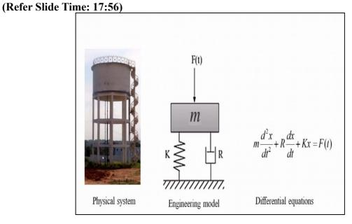
So let us assume that this physical system that is the water tank is located in area where very high speeds winds do occur, so we want to study these physical systems. Now you can see that this physical system is composed of a lumped mass or say the mass of the water tank and there are pillars and these pillars essentially behaves as speed.
