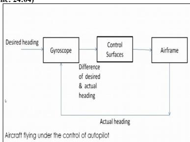
We can take an example of the system as saying a simple aircraft flying under the control of autopilot. So, if I take this system then there could be various sub components of this system,
