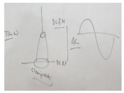
So if we see here like the process like GT welding or GTW process where use of straight DCE and polarity producing the lesser heat and more heat in the work piece site, while if the DCRP is used, in that case we get the much better cleaning action. So these are the two contracting requirements, we want that less heat is generated in any case for the much better life of the electrode.
