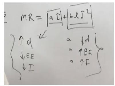
That is what we will try to talk about here. So here, if we see a is the coefficient or the constant, which accounts the voltage drop in the anode drop zone or cathode drop zone, the chemical composition and the factors all those material and process related factors that are affecting the heat generation due to the heat generation in anode drop zone or the cathode drop zone. I is of course the welding current in ampere.
