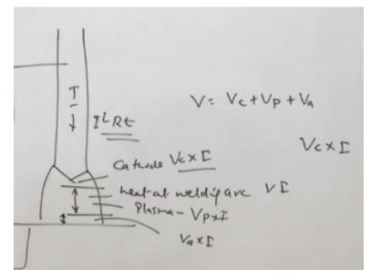
The fundamental aspects, which I want to take up first, they are related with the factors governing the melting rate in case of the arc welding process and for this purpose, what we have to see, the one empirical equation, which have been developed like aI + bl I square, where there are two terms, which in combination determine the melting rate and what these two terms are all about.
