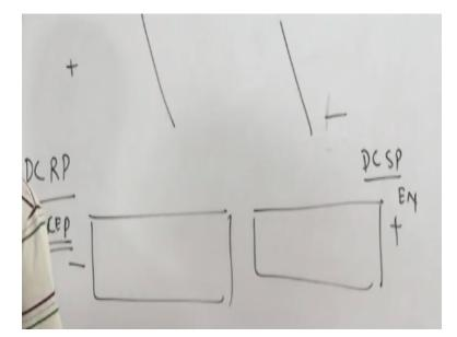
Like the electrode and work piece can be connected either to the positive or negative terminal or in case of AC, of course, these two will keep on changing. So when the positive terminal is connected to the electrode and negative to the work piece, in this case what we say, the DC reverse polarity where your work piece is negative and the electrode is positive.
