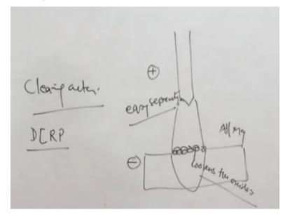
Like say this is Tungsten electrode or any other process electrode, like say in this case if the aluminium or magnesium, if they are welded using the GTW process making the work piece, negative and electrode positive. So in this case our work piece is expected to emit the electrons and if the mobile cathode spot is formed, the surface of the work piece, so mobile cathode spot formation actually loosens the oxides being formed.
