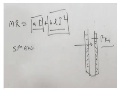
For example, in case of the shielded metal arc welding process, higher level of the current is limited by the situation or by the current value, at which thermal decomposing of the coating starts due to the flow of current, say this is electrode and this is the coating. If you keep on increasing the current value, then high I square or heating of the core wire can start damaging the coating much earlier than it should.
