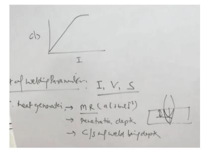
Now coming to the effect of welding parameters. There are 3 welding parameters, which are extremely important and determine the kind of joint, which is produced and these are like welding current, voltage and welding speed. So what we have to see, we know I directly affects the heat generation. Because the arc welding is a high current and low voltage process. So if the current is changed, then it affects the heat generation significantly.
