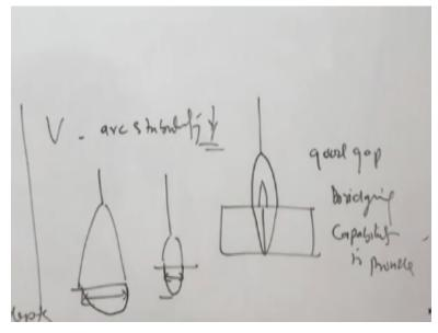
On the other hand, if we see the voltage, voltage does not play big role in generation. It contributes, but effect is not that high as that of the welding current, but it certainly affects the arc stability. If the arc voltage is not enough, that it will lower the stability of the arc. We know that if we see that, if the arc gap is short, then the arc voltage is very limited. Under identical conditions, if the gap is increased, then arc voltage increases.
