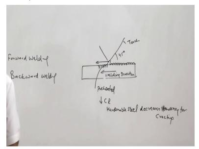
So you know the as far as the gas welding is concerned gas welding is performed using two techniques like forward welding and backward welding, forward and backward welding these two names come from the orientation of the - the welding torch with respect to the welding direction, if this is the welding direction and then torch is pointed at about 45 degree and the tip of the or you can say the torch nozzle off the torch is a point in towards the direction of the welding in this case.
