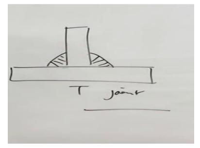
Tee joint is the simple one where the one plate is kept in horizontal position and another member to be join is - is brought somewhere in between at 90 degree and then fillet weld is made to make the tee joints, so this is you can say the tee joint so that is how they are 5 types of the weld joints butt, lap, corner, edge and the tee joint and the welding positions four the flat welding have explained already, horizontal welding, vertical welding and the overhead welding.
