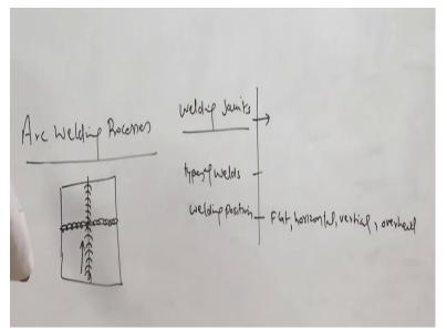
So in this case like say this is the vertical plane and the weld metal deposition is also vertical, so it can be moving down or it the position can be in up fill manner like moving up, so both types of the movements are used for depositing the weld metal, its - it is difficult to deposit the weld metal in both vertical as well as a horizontal position and further more difficult position is the overhead.
