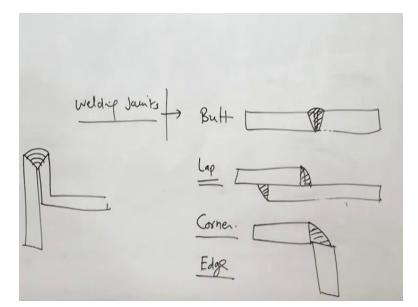
Now coming to the types of the welded joints types of the weld joints are like butt joint when the plates to be welded or kept in butting position means they are in and two ends are matched with each other, it may be square or it may be a V or W, double V, single J, double J like that and different types of geometries are there, so the plates to be welded or kept in butting or and two end touching positions and then joint is made.
