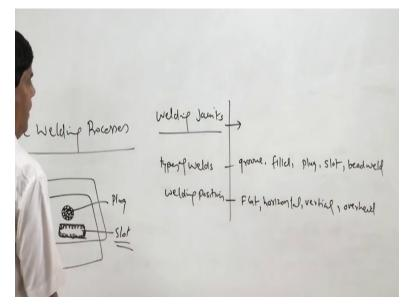
In case of the plug and slot, the plates are kept in like say the two plates one in the in top view if we see and this is the another plate and the two are to be joined then what we do we make as a hole in the upper plate and then the weld metal is deposited like this when the fusion of the lower plate is also achieved. So basically hole is made on the - on the upper plate.
