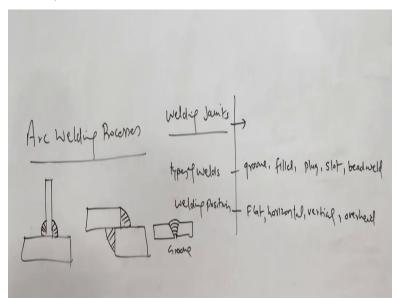
Then types of the weld like one is the groove weld, then fillet weld, then we have like plug weld, slot - slot weld and bead weld - bead weld. So the groove welds are simple where either the square joint the - the groove is made at the faying surfaces or then the weld joint weld metal is filled in this is called groove weld.
