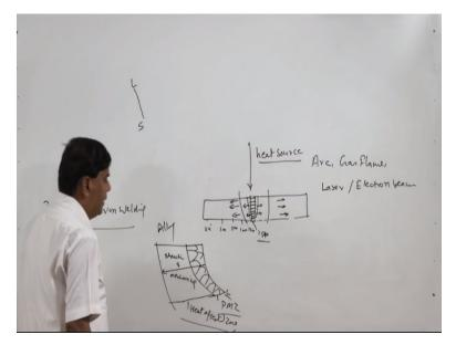
So due to the thermal conductivity of the base metal, some of the heat is transferred to the underlying metal below the fusion boundary and this heat transferred to the base metal increases the temperature of the metal to the different degrees, say here it may be 24 degree, then 100 degree, 500 degree, 1000 degree likewise say 1200 say 1500 in case of the steels or 1540 degree centigrade.
