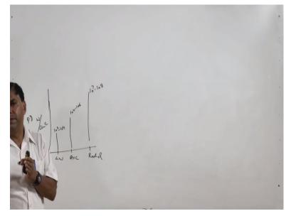
I have told in the last previous lecture, I have told you that the guess welding, arc welding and like say the radiation welding like laser and all these are in increasing order of the power densities, like say 10 to the power 7 to 10 to the power 8, 10 to the power 4 to the 10 to the power 6 and like say 10 to the power 3 to the 10 to the power 4, power density in terms of watt per centimeter square.
