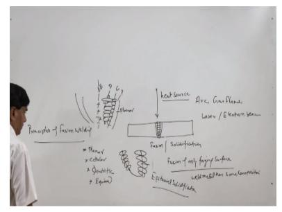
So basically the principle of fusion welding that is what we have to talk. Like the components to be joined after proper cleaning of the faying surfaces using suitable heat source, heat source is applied in form of arc or gas flame or like say the laser or electron beam and likewise any other heat source, so this will be directed onto the surface, faying surfaces of the component primarily to bring them to the molten state.
