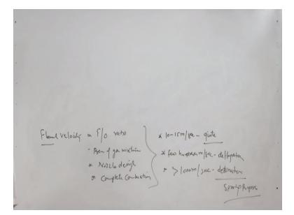
Now depending upon the flame velocity, flame velocity depends upon the fuel and oxygen ratio and the pressure. Pressure of gas mixture being used for the combustion purpose and the nozzle design, etc. and how effectively the combustion, how effective complete combustion is taking place. These are the four factors that will govern the velocity of the flame.
