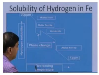
Now, we will be going into the mechanism and the causes of the cracks. So here we will see that the solubility of the hydrogen in the well, in the liquid state and the solid state is different. Further the solubility also, solubility of the hydrogen in the iron changes with the temperature due to the change in the crystal structure or due to the change in the phases, which are observed.
