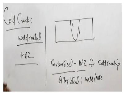
So this kind of crack can occur either in the weld metal if it has a favorable conditions like the martensitic structure, high tensile residual stresses and higher concentration of the hydrogen as well as the higher hardness. So the weld metal or it can also occur in the heat affected zone. It is commonly observed in the heat affected zone. Now coming to the kind of metal systems, which are sensitive for such kind of cracking.
