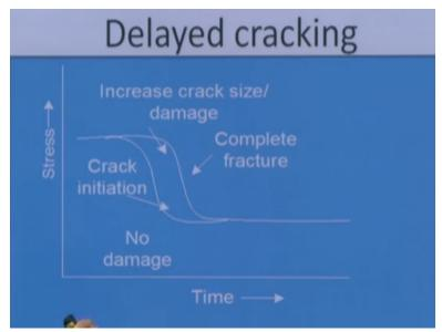
So the delayed cracking is the time based cracking, where it takes time under the different level of the stresses and the hydrogen concentration. This typical diagram shows that how the cracking starts and how it ends and leads to the fracture. So as a function of the stresses that may be tensile residual stresses or the external stresses, as a function of time, if we see, if the stresses are high.
