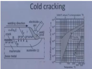
So what happens in case of the welding due to that, this difference in solubility? Let us say we, this is the direction of welding and this is the region next to the weld metal and this is the base metal. So base metal, of course will have the ferrite and the iron carbide. But whatever region falling in the weld metal zone or next to the fusion boundary that will be falling in the heat affected zone.
