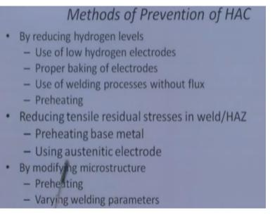
These are the prevention methods. As I have explained earlier, reducing the hydrogen level, using the low hydrogen electrodes, proper baking of electrodes or use of the welding process, which are without flux or preheating. All these things I have already explained for reducing the hydrogen. And reducing the tensile residual stresses in the weld metal, as I have said, use of austenitic filler or the preheating of base metal also helps to reduce the magnitude of the stresses.
