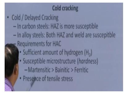
So if we see here, these what I have already said, in the carbon steels, HAZ is sensitive for the cold cracking, while the alloy steels has, in case of the alloy steels both HAZ and the weld are susceptible for the cold cracking. And so for development of the cold cracks or hydrogen assisted cracks, it is necessary that there is sufficient amount of hydrogen, susceptible microstructure, sufficient hardness.
