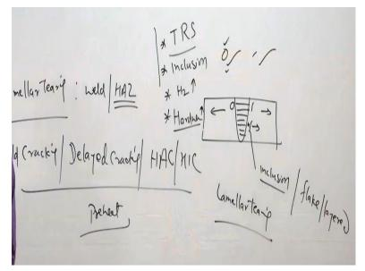
First, the Lamellar tearing is one kind of the crack observed both in the weld and the heat affected zone. But the formation of this kind of the crack or tearing is more commonly observed in the heat affected zone and another one is called as the cold cracking also known as the delayed cracking, also termed as the Hydrogen Assisted Cracking or Hydrogen Induced Cracking. These are the four different names which are given to another type of the crack which is observed in the heat affected zone.
