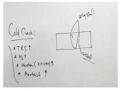
So this is common for the carbon steels and in case of the alloy steels both as well as the heat affected zone for the alloy steels. The things that are needed for such kind of cracking is like the presence of the tensile residual stresses, one, hydrogen concentration, two, so all these will be promoting the cracking tendency and the 3 higher hardness, a hardness greater than 350 VHN actually promotes the cracking and the sensitive structure like martensite.
