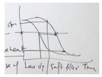
This diagram goes in like this. So this is the time and here we have stresses. So for any magnitude of this stress, this is the time when the crack will, the hydrogen crack will initiate and hydrogen induced crack will initiate. And this is the time when cracking will complete and the fracture will start. So higher the stresses, lesser the time it takes for complete fracture or initiation of the crack and lower is this stress, greater is the time it takes to.
