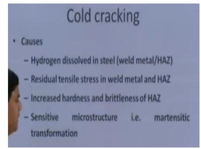
These are the common causes, which are observed for the development of the cold cracks. Hydrogen dissolved in the weld metal, hydrogen dissolved in these steels like in the weld metal or in the heat affected zone, development in the tensile residual stresses in the weld or heat affected zone, higher hardness or the brittleness of the heat affected zone and the crack sensitive structure like the martensite formation in the heat affected zone.
