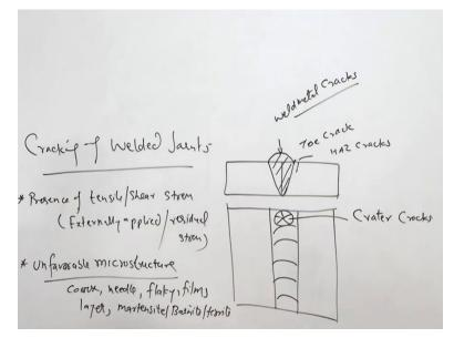
And it includes say the presence of the - presence of the tensile or shear stresses, these stresses may be externally applied - externally applied or this may develop due to the differential expansion and contraction during the welding so leading to the development of the residual stresses, so this also promote the cracking under the favorable conditions of the weld joints and third is favorable - favorable micro constituents micro structure.
