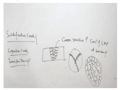
Another one is the refining the grain structure, if the grain structure of the weld metal is very coarse like this then - then it will be leading to the segregation of the alloying element at the center more segregation at the center as compared to the case when the grain structure is fine, so basically the coarse structure increases the concentration of the low melting point impurities at the boundaries or the grain boundaries.
