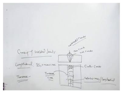
Longitudinal crack like the solidification crack is a typical example of the - the longitudinal crack, the cracks which are run parallel to the welding direction or the cracks which are next to the fusion boundary running along the welding direction parallel to the welding direction also can be termed as the longitudinal cracks, so normally crack - cracks in the HAZ running parallel to the welding directions can be termed as the transverse cracks.
