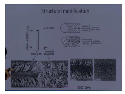
Now we will see that these are the typical methods which are used here like when there is no arc acceleration the grain size the crack length we will see the solidification cracking tendency the crack length is more and when the arc oscillation is implemented it refines the grain structure and modifies the grain structure and which in turn reduces the - the - the crack length which is observed of - after the welding.
