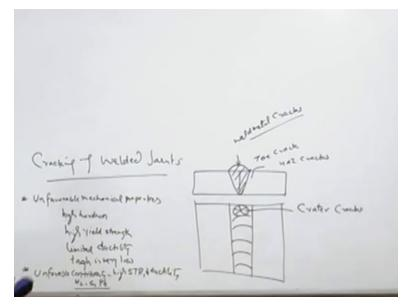
So we will start with the - the cracking of welded joints and the different types of the metal systems are found sensitive for the different types of the cracks which may be in the either heat affected zone or in the weld metal. So let us say the component like this joint using the fusion welding process, so in this case we may have cracks in the different locations which may be here like the toe of the weld in form of toe cracks - toe crack.
