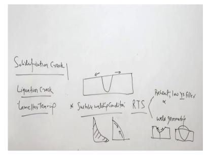
So these 3 approaches they work on the different concepts, the first one is like favorable or suitable welding condition, so that the residual tensile stresses can be reduced and for this purpose the approaches that are used, one is like using preheat so that the expansion and contraction is by enlarge differential expansion and contraction can be reduced in order to develop - in order to reduce the development of the residual tensile stresses.
