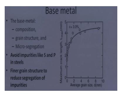
This is what we can see here when average grain structure, average grain size is less than the crack length is also less, while the when the grain size is increased it increases the cracking tendency at the same time the presence of the impurities in the base metal like sulphur and phosphorus also need to be avoided and we need to refine the grain structure so that the segregation tendency of these impurities in the - in the base metal can be reduced.
