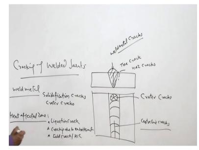
So but we will see that the specific types of the cracks and what are the reasons for their developments, so as I have said the broadly there are two locations the cracking in weld metal and cracking in the heat affected zone, so cracking in the weld metal in this category mainly we have the solidification crack which significantly - significantly - which significantly important because it leads to the rejection of the joints.
