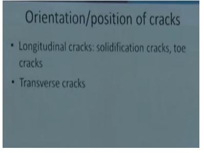
So orientation or position wise cracks, longitudinal crack say like solidification crack or the transverse cracks. So now I will take up the 3 types of the cracks one by one and what can be done to overcome the reduced tendency of development of such kind of cracks, so these 3 cracks are the solidification cracks, liquidation cracks and the lamellar tearing which is observed in the heat affected zone. So starting with the longitudinal sorry solidification cracks
