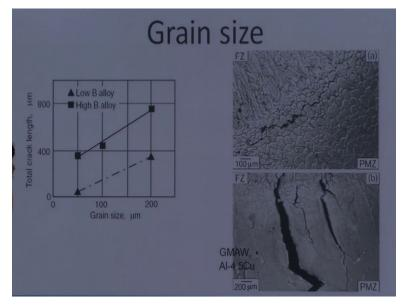
So here it shows the typical way by which the - the grain structure affects the cracking tendency, so when the grain size is fine the crack length is limited and the grain size is large the crack size is more this is what we can see here this is weld zone this is a base metals side, so this is the area
