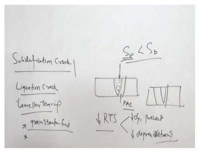
So the one of the points means one of the ways of reducing the cracking in the liquation liquation cracking in the PMZ region or partial melting zone is to reduce the residual tensile stresses for which we can use the low yield strength filler or we can use preheat or we can reduce the degree of restraint - degree of restraint, so all these approaches will help to reduce the magnitude of the residual stresses being developed.
