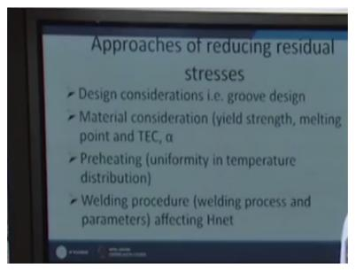
Design considerations, we try to select the weld joint groove geometry in such a way that the volume of the weld metal can be reduced so the residual stress development can be reduced. The filler metal is selected in such a way the yield strength is low, expansion coefficient is also low. So that the related expansion and contraction can be reduced and the maximum magnitude of the residual stress can also be reduced.
