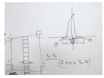
Like the two plates being welded under the restraint conditions with both the ends, all four corners and the weld joint is made between these. So obviously they will be expanding during the heating and contracting during the cooling. So this expansion and contraction will be leading to the development of the residual stresses. So this is the length of the weld, which will be shrinking from the melting point to the room temperature.
