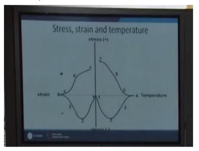
And if we try to study the way by which its temperature raises and how the strain and stress it experiences, here this side shows the strain, stress positive, stress negative and the temperature. So when there is increase in temperature, first the negative compressive strain is experienced. So initially the compressive strain due to the increase in temperature increases. Thereafter, softening starts.
