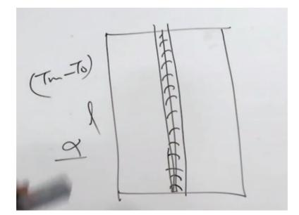
Let us take the two plates like this when the weld is made like say length is 1 and the temperature melting point to the room temperature T naught and alpha is the expansion coefficient and this is the length of the weld, which is made assuming that entire weld is made in one go which will be shrinking on cooling from melting point to the room temperature.
