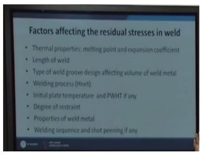
And then the properties of the weld metal lowly strength weld metal is always favorable from the residual stress point of view because that will help in reducing the residual stress magnitude, post weld heat treatment like stress relieving and the shot peening helps in reducing the residual stress magnitude. Apart from these there are other various factors that will be determining the residual stress magnitude.
