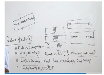
Another is the weld joint design, this factor is basically related to the kind of groove, which is being used. It is the square or V, U or J or the double V, double U, J (()) (21:14) etc. There are various types of groove geometry and purpose of all this is to see that because the groove geometry affects the volume of the weld metal. So any geometry, which is increasing the volume of the weld metal.
