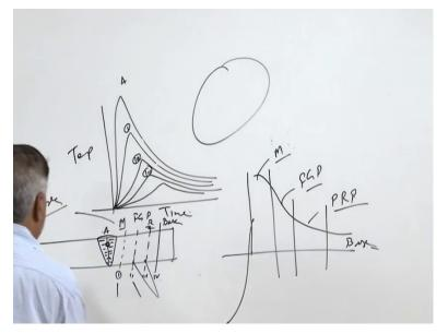
So in general if we plot the variation in the hardness as a function of the distance from the fusion boundary than typically in the weld joints in the simple carbon steels the variation like this is a fusion boundary what we will see that as a function of the distance from the fusion boundary we say this significant higher hardness and then hardness will keep on decreasing so this high hardness is attributed to the martensitic transformation.
