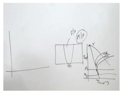
So far we have not talked about the weld, in general weld experiences the much higher heating rate as well as cooling rate and that is why as per the carbon content in the steel mostly it forms either ferrite or pearlite or it may form the martensite and the pearlite in the weld and that is what will be governed by the composition of the steel, so for that we need to see the CCT diagram for the - for that particular grade of the steel.
