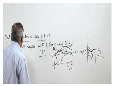
And this variation is attributed to the changing proportion of the ferrite and pearlite which are formed normally, if we will see like 0% carbon content 0.8% carbon content and 1.2% carbon content in x-axis and here is schematically if we show the structure in the first half say 100%, so here we start it will go in like this so here this shows the ferrite content when the carbon content is 0 the entire system is ferritic and the pearlite is 0.
