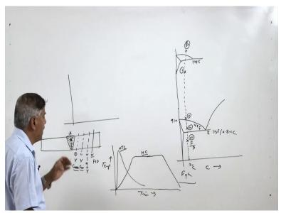
So in case of the carbon steel we see - we know that which kind of the phases which will be formed during the welding that will depend upon the kind of the weld thermal cycle being experienced by the different zones, so if we will see let us take this example where the two plates are being welded - are being joined by diffusion welding process, so the weld zone is produced from this metal is brought to the molten state and thereafter solidification proceeds.
