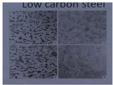
And this is what the actual diagram shows in the - the base metal having the - the light touched white ferrite ferritic grains and the dark edged the pearlitic grains when they are heated to the point 2 like this one heated to the point 2 and then cooled rapidly then it results in the partially refined zone.
