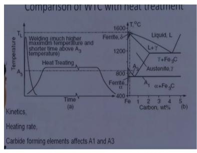
This is what I have already explained that, there is a lot of difference in terms of the weld thermal cycle and the heat treatment cycles which are used for the two cases.
