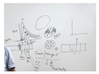
So if we see again another case like this the heat affected zone, so here in this area if we have if the weld thermal cycle is such that enough time is not available for homogenization of the austenite, so the and carbon is not able to diffuse equally in the entire mass to have the homogeneity in terms of the composition.
