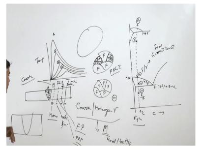
For example here as per the according to the weld according to the iron carbon diagram it should - it should be like at point 2 it should be the homogeneous fine austenite, it should be the homogeneous coarse austenite at point 1 and it should be austenite and the ferrite at the point 3, but since during the welding the weld thermal cycles being experienced at the different points are completely different like this say for point A.
