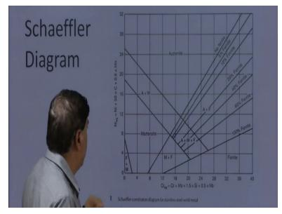
Schaeffler diagram is basically shows its diagram which shows the effect of the composition on the kind of phases which will be formed, so this diagram has the two axes, one is the x axis shows the chromium equivalent and y axis shows the nickel equivalent, so chromium equivalent means it is the sum of the all those variety stabilizing elements like and how it is obtained the chromium nickel comprises chromium + molybdenum + 1.5 multiplied by silicon + 0.5 of the niobium.
