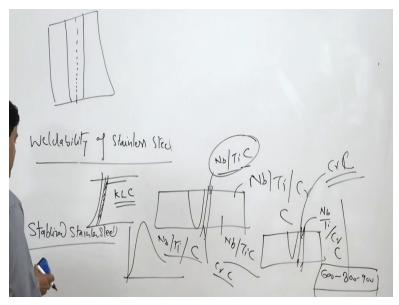
But under the different kind of the circumstances to understand that we will quickly see this diagram this one will be having say niobium and titanium of course it will have carbon and chromium, so whenever the weld is made so the regions very close to the fusion boundary where in the niobium, titanium all these carbides will be decomposing, while that location away from they will not decompose and they will have the niobium or titanium carbide stable.
