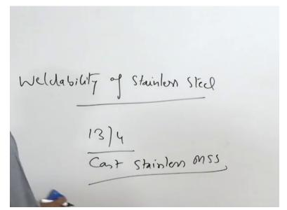
One typical use of the cast stainless steel is like making the - the turbine components in hydro turbine components typical 13 4 cast stainless steel is used this - this primarily becomes the martensitic stainless steel, because of its very good combination of the hardness strength and toughness its is used for making the hydro turbine components primarily these are used for making the blades.
