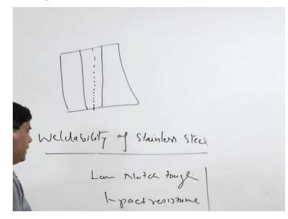
And such kind of intermetallic phases whenever they form or loss of no toughness and impact resistance, these two are very badly compromised and that is why their formation is avoided during the welding of the austenitic stainless steel, apart from the similarly the problems are also associated with the ferritic stainless steel and martensitic stainless steel. Ferritic stainless steel primarily experiences the problem of loss of toughness in the heat affected zone due to the grain coarsening.
