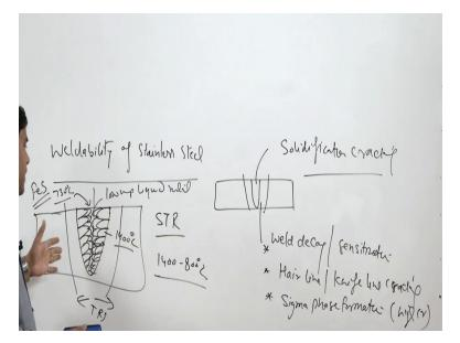
As far as since these steels are used for fabrication of the various engineering components which require welding that is why the weldability of these steels become of the great importance, so as far as the austenitic stainless steel is concerned - austenitic stainless steel is concerned the common problems which are encountered during the welding of the austenitic stainless steel are of the two categories.
