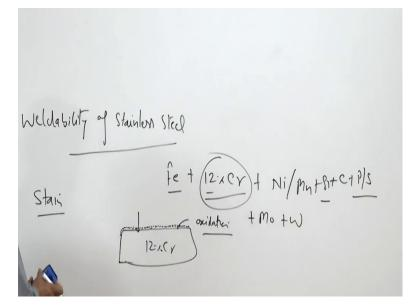
So if you have to talk about the weldability or is of welding of stainless steel then we need to first know a little bit about the stainless steel themselves, the stainless steel are basically these are iron based system where in chromium is normally added more than 12% and this presence of the chromium in steel apart from chromium there is other alloying elements like nickel or manganese + silicon + carbon, phosphorus and sulphur.
