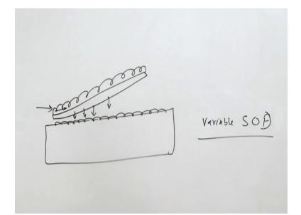
There is another situation where in sometimes in special cases if you want that impact of the prime component with the main component does not takes place in one go in that case especially the - the prime component is placed at an angle like this and this is the main component say to which the prime component after the impact, so there and over this we can and have either buffer plate or we can place the explosive over it like this.
