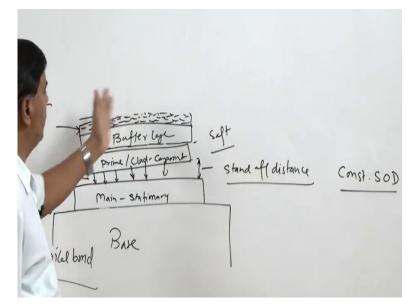
So here we will see very robust base is used which can sustain the heavy impact so which is created by the explosion, so the component to be welded is the component there is the one main component which you can say main component to which joint is to be made, so this is stationary it is kept on the base and another component which is to be joint is made the prime component like this it may be a cladding material or it may be another member.
