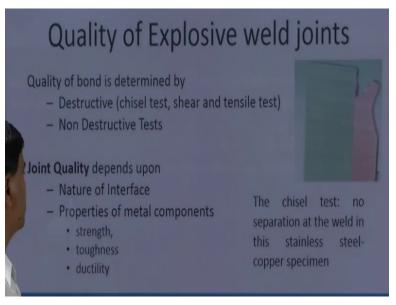
In case of the stainless steel copper joint say this side we have copper, this side the stainless steel and chisel test is conducted, so this in the interface is still intact but the failure starts from the copper side, so this is one typical test which is and the unique one and mostly accepted for that explosive welded joints.
