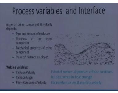
Thus so if we see here the angle of - so the - the angle at which prime component is replaced and the velocity at which it should impact depends - this will depend upon the how much amount of explosive and the type of explosive has been placed greater the amount and explosive of the higher energy will be offering the greater impact velocity.
