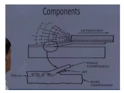
This is what we can see here, this is how the collision - the ignition starts and it propagates from one end to another and this is the we can say in this portion already the explosion has taken place or detonation has taken place and with the impact the prime component has impacted with the base metal and it has been welded and this is what in enlarged view we can see the prime component in the upper one and the base component lower one.
