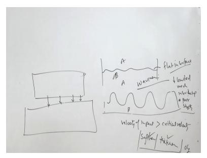
Normally, when the let us say this is the prime component and this is the main component after the explosion prime component impacts with the surface of the base metal, so after the impact sufficient heat is generated huge impact causes the plastic flow of the material at the interface and this in turn causes the interface of the wavy in nature like this, so this kind of nature like this side A metal and this side B metal.
