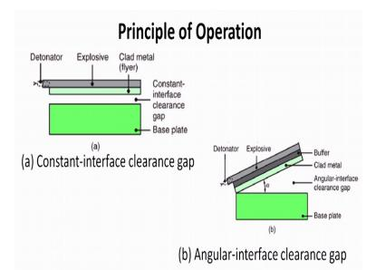
The cladding material or the prime component and the base component the constant interface clearance, in this case constant interface clearance gap or the constant standoff distance, in another case the buffer layer is placed in between to avoid any kind of erosion to the prime component or the clad material which is placed at certain angle is called angular interference clearance gap and then base plate.
