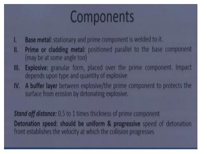
So if we see there are 4 components basically, the base material which is kept stationary over the anvil and the prime component which is welded and kept at the top prime component maybe another member or it may be in form of the clad material, the prime component or the clad material is positioned either parallel to the base component or it may be kept at certain angle depending upon the requirement.
