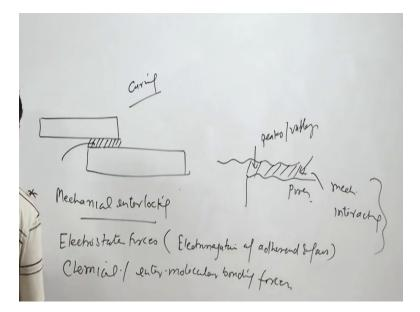
So the three mechanisms are - are there they can work interdependently or the - the role can be interdependent and they in combined way also they offer the strength of the adhesive joint, one is the mechanical interlocking, mechanical interlocking basically uses the concept of like all the surfaces will have the - the ups and downs over the surfaces. And when the adhesive is placed it will be filing the peaks and valleys present at the surfaces.
