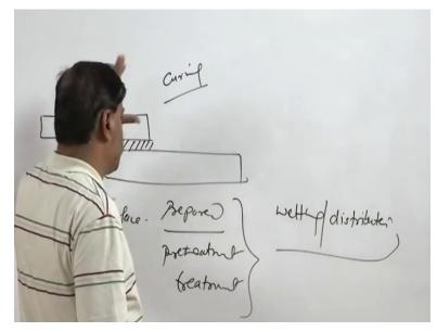
So if you see the how adhesives work like say the members to be joint maybe of the same or the different types when so the first step is that all faying surfaces - faying surfaces are properly prepared preparation is done for to take to remove all impurities like oil, grease, dust, draught etc. from the surface so the surface is prepared and then it is subjected to the pretreatment so pretreatment further help to avoid the oxides, observed gases moisture etc. from the surface.
