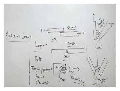
So the common the joints which are made in lap joint configuration and butt joint configuration and there is tongue - tongue joint configuration which is tongue and groove joint configuration, so these are the three, apart from this the some of the joint configurations which need to be avoided includes the peeling situation and the cleavage situation the kind of the loading which adversely affects the capability of the adhesive joints.
