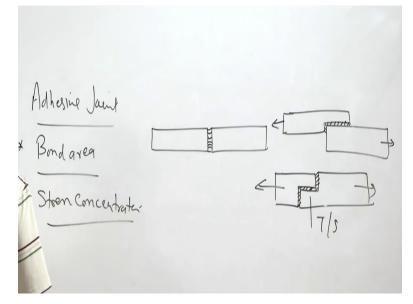
Then we will see the for butt joint configuration the common one is this one but since it offers somewhat lesser the bond area so to increase the bond area like this this is the typical common one, but it is modified in the two ways one is the simple sheet is kept like this and another sheet is prepared this manner, so that the plates and here this area is applied with the - the adhesive bonds, so this is another modification say for the butt joint configuration.
