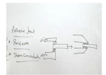
So this is how we can increase the - the bond area as well as reducing the stress concentration, there is one more way to increase the load carrying capacity where in the double sided plates are used, like say this is one plate and then what will be doing another plate is brought in like this, another one is brought like this and between the two the bond is made from the two sides so this bond this is one load carrying capacity and this is this one member.
