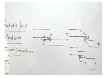
One is our bond area is really large enough and the second is stress concentration is very limited, because it can start the separation at the interface of the adhesive and the sheet being joint, so these are the two factors are kept in mind and therefore considering this in mind the joint configurations one is the simple one, in the lap joint configuration joint area that is the overlap length is selected in such a way.
