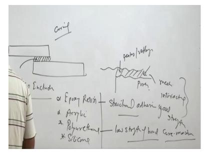
So and apart from this the common adhesives which are used to for the purposes of the adhesive bonding, so includes adhesives includes like epoxy resins this is one, acrylic is another and we will have there is one or two - one or two more adhesive which are commonly used is like polyurethane and silicon. So these are the common adhesives, epoxy resins is a very common structural adhesive which offers very good strength.
