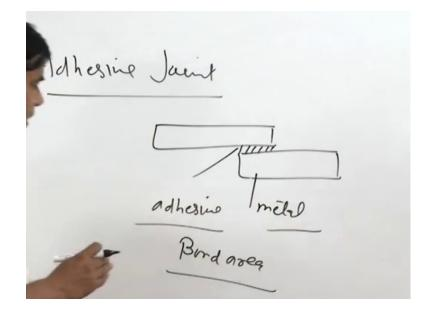
In addition to this, for designing the adhesive joint what we have to keep is adhesive joint design what it includes basically we have like say the members to be joint and what we have in our hand is this the adhesive can be placed between the faying - between the members to be joined since the - the mostly the metals offer much higher strength than the adhesives, so adhesives being weaker than the metals.
