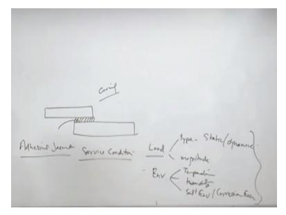
So apart from this for achieving the desired joint or adhesive joint with the desired properties must be designed properly, so the design of the adhesive joint depends upon the service conditions whatever design is there that should satisfy the service conditions and service conditions mainly include the load in terms of the type let that is static or the dynamic and then magnitude the magnitude of the load.
