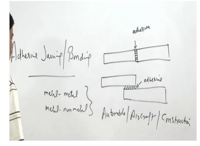
So here the topic goes in like this adhesive joining or this also known as adhesive bonding, so as name reflects that the components to be joined or kept mostly either in the butting position like this or they are kept in the overlapped position, so mainly the lap joint or the butt joints are made and between the - the faying surfaces adhesive is applied. So adhesive is applied and here this is an adhesive.
