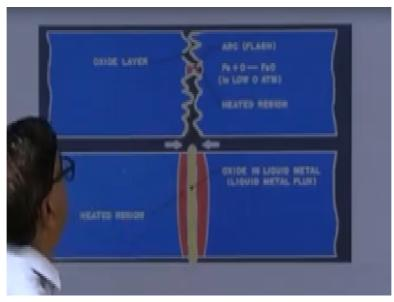
And we will see this is the what happens actually at the interface. In the initial stages when there is a contact through the peaks and valleys, so there is a heavy flow of current. The peaks and valleys causes very localized heating. And the oxide layer will be getting heated and when this happens means the arcing and sparking continuous for long it results in the layer of the molten metal wherein having the oxides.
