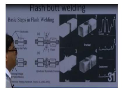
So here we can use this also schematically the four stages have been shown here. Initially in the initial stage, the parts to be joined are kept on the two clamps of the copper shoes, with the proper position. So, in the initial stage this is the position when they are brought together. Initially like say initially, we may have may have pre heating or may not have so in case of preheating entire the ends of the work piece are heated well.
