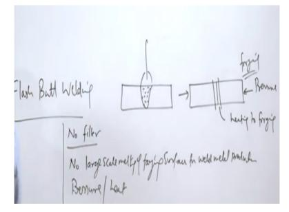
The kind of temperature which is needed for this purpose with each like preheating through I square RT heating and the heat generation due to the arcing both these have their own specific role for a development of the joint like since this process is a one variant of the solid state process also. So as the joint is not formed in DES by melting the faying surfaces of the base metal, but joint is forging the components to be joined together.
