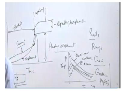
Now we will see the kind of variations which takes place during the welding in respect of the time and the pressure. Time and the pressure, so. Here this will be showing displacement. Displacement is about kind of movement here work piece and this is the another work piece. So how the movable and moves towards the; movable work piece moves towards the fixed end so that the magnitude keeps on increasing.
