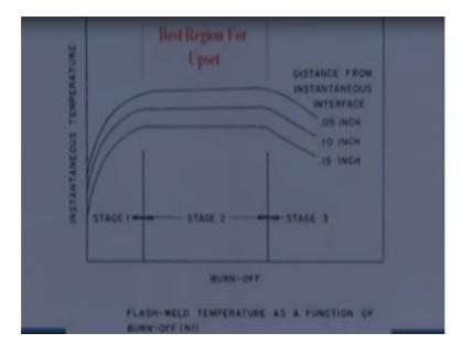
So, this what will see that the different stages which are being shown. In the initial pre heating stage, in this stage one, there is a flow of current. In the pre heating stage, there is a continuous rise in temperature. And then temperature remains constant in the stage two. And once the flashing is over upsetting starts. The temperature starts coming down. As the function of the time or this is also the burn off period.
