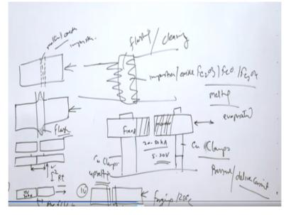
So, this is what is there in the basics of the process. As a whole how does it work in that is what and now we will let you know in detail. So, this process in this process one work piece for the members to be joined. Say one piece is kept fixed like seaweed, be helped off the copper supported clamps copper clamps and another end is kept a moveable, say this is a movable part or another work piece to be joined, which is kept moveable.
