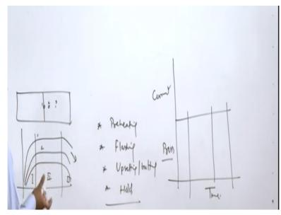
So, the interface like this. If this is the interface, point 1, point 2 and point 3. So, the kind of variation in temperature, the temperature will be higher. At 1, the temperature will be somewhat lower, at 2 and at 3 like this. So, in the stage 1, stage 2 and stage 3. This is the upsetting stage,
