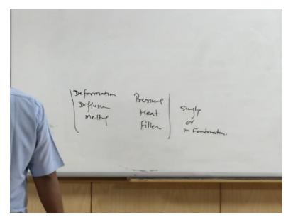
Since the deformation, diffusion and melting these are the three things which are there they will use pressure, heat and filler either singly or in combination. So, using these three fundamental aspects the different range, very wide range of the processes have been developed over a period of time. So, over a period of time we will see that very large range of the solid state joining process, very large range of the solid liquid state process and the liquid state process have been developed.
