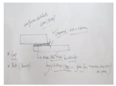
As far as the process principle is concerned and the process is concerned here, what we will do the components mainly the two types of the joints are made, the most common one is the lap joint configuration and sometimes even butt joint can be made for those cases, but for making the butt joint, sometimes beveling is in which especially tried so that the required joint strength can be achieved.
