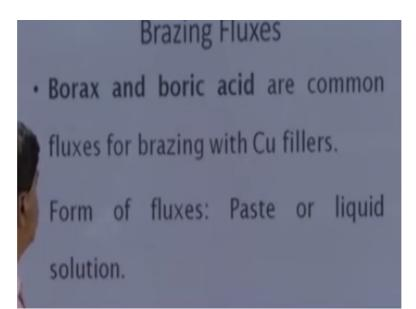
The common fluxes which are used are borax, boric acid and these are, the fluxes commonly used with the brazing for the brazing purpose with the copper fillers and thus these fluxes can be used in form of paste or the solutions or the powders, they can be applied over the surface. So now here I will conclude the presentation.
