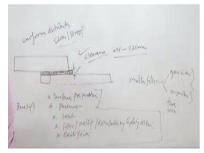
So here as far as the steps are concerned, first the surface preparation with the proper cleaning preparation. The second is the placement with the proper gap. Third is application of the heat, then the filler is brought to the molten state melting and then distribution by the capillary action and there followed by the solidification. Once the solidification is completed, the joint is prepared or joint is ready.
