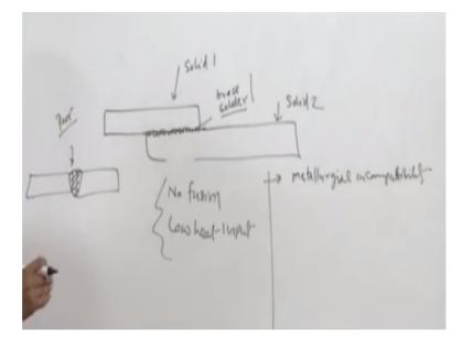
Why are these called so because the base metals to be joined are kept in solid state means, they remain in solid state like 1 and solid 2. While the material which is used for developing the joint between these two is brought to the molten state, which is called either called braze material or solder as per the kind of the process to be used. So brazing material are the solder.
