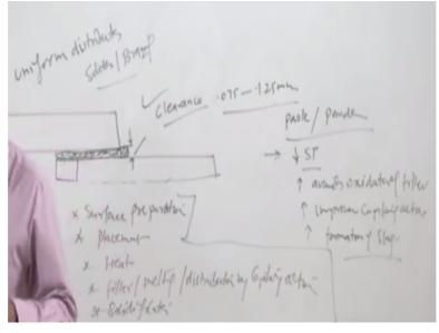
So fluxes are also applied or placed before hand when the filler metal is placed so that the flux also melts along with the filler metal and it works effectively in number of ways. so the application of the flux namely may be in form of like paste, powders which is applied and then this flux after melting does number of things like it lowers the surface tension of the filler metal, it avoids the oxidation of the filler.
