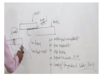
Another is those metals which have the poor weldability means they can be fused but when the joint is made, the kind of properties that we obtain are poor like this, the two components to be joined having the poor weldability when they are fused either it will result in lot of ferocity in the weld or cracks in the weld or in the heat affected zone.
