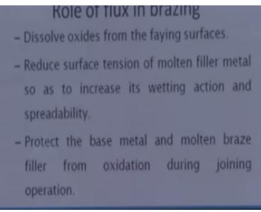
The fluxes help to dissolve the oxides from the faying surfaces, reduce surface tension in order to improve the fluidity and these protect the base metal and the molten braze filler metal from the oxidation during the joining operation.
