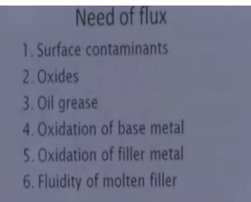
These are the different purposes for which fluxes are used. It takes care of the surface contaminants, oxides, oil grease, oxidation of base metal, oxidation of the filler, and fluidity of the molten metal. The oxidation and the grease and oxides and contaminants are taken care of while the fluidity is improved by the filler.
