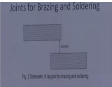
So the clearance is extremely important for having the capillary action in order to ensure the uniform distribution of the filler material between the faying surfaces.
