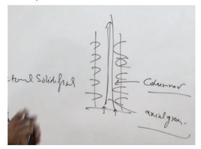
Directional solidification means the process like it starts from one end and then it completes at another end. Of course the columnar grain structure appears from both the sides of the plates being welded but sometimes axial grains are also observed running along the weld line. So, there are two types of the grain structures are normally observed one is the columnar grain structure which will be perpendicular to the faying surfaces of the base metal and another are the axial grain structure.
