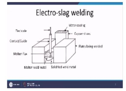
So, here if we see this is the process. This is electrode fed which is, electrode which is fed through the automatic roller feeders normally constantly speed kind of speed drives systems are used in this case the electrode is fed and it is fed through the contact tube or guide tube. This guide tube will be feeding the electrode down to the bottom. These are the two plates is one another plate but this is the front view you can see and these will give us the top view.
