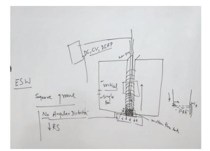
So, if you see the joint is square grove type. So, what all sink it takes place that is symmetrical and symmetrical transvers shrinkage of course it is there but in this situation there is no angular distortion. There is no angular distortion in this case and the slow cooling conditions, high heat input and symmetrical shrinkage results in the reduced residual stresses. Now, we will go further in to the details of the process especially when we are working with the heavier plates.
