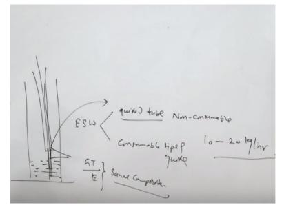
So if the gap is really if the height of the plate to be welded is really very large then the long electrode must be fed through the guided tubes. So these, there are 2 variants in this process, electro-slag welding come with the welding process come with the 2 variants, one is where guided tube or guiding tube which guides or fits the electrode in particular path it is a non-consumable kind, it is not consumed.
