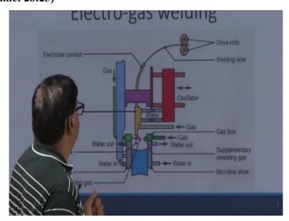
So, that is what we will see here. In this arrangement here like say these are the plates to be weld, these are the copper shoes and here we see copper shoes fed with the water. Water comes and gets into the copper shoes and then it comes out and this is where the weld is being, this is weld metal and will see that is this is the spool where from the, this wire feed drive system and the wire is fed through the spool.
